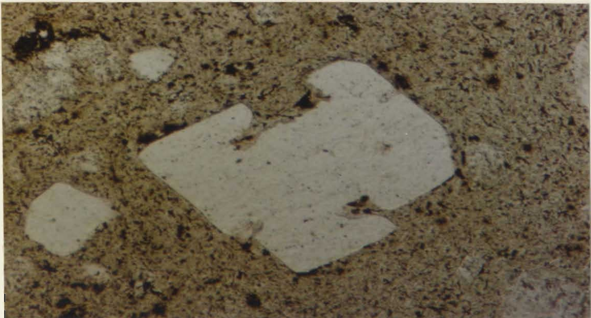
Plate 22: Photomicrograph showing euhedral quartz with embayed boundaries in the St. Lawrence granite (plane light). Thin section no. 94. Field of view 2 mm. by 1.3 mm.
