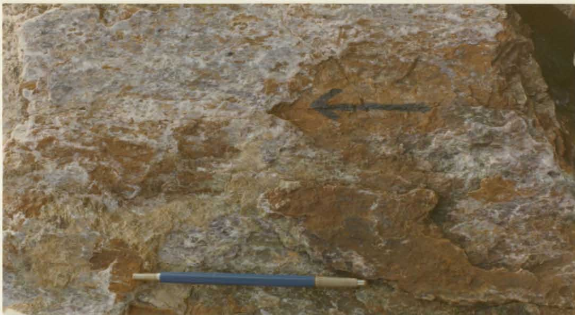
Plate 23: Slickensided surface coated with red hematite and purple fluorite at Little St. Lawrence quarry.
