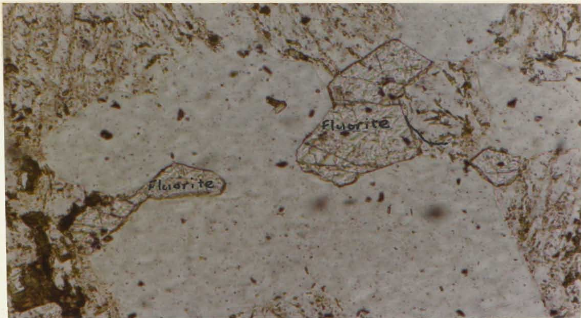
Plate 21: Photomicrograph showing fluorite crystals as accessory minerals in the St. Lawrence Granite (plane light). Thin section no. 142. Field of view 1 mm. by 0.6 mm.
