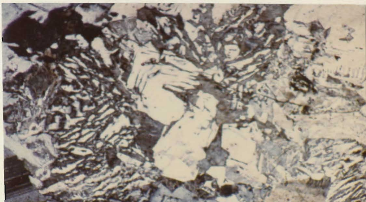
Plate 16: Photomicrograph showing granophyric texture in the St. Lawrence granite (cross-nicols). Thin section no. 3. Field of view 2 mm. by 1.3 mm.
