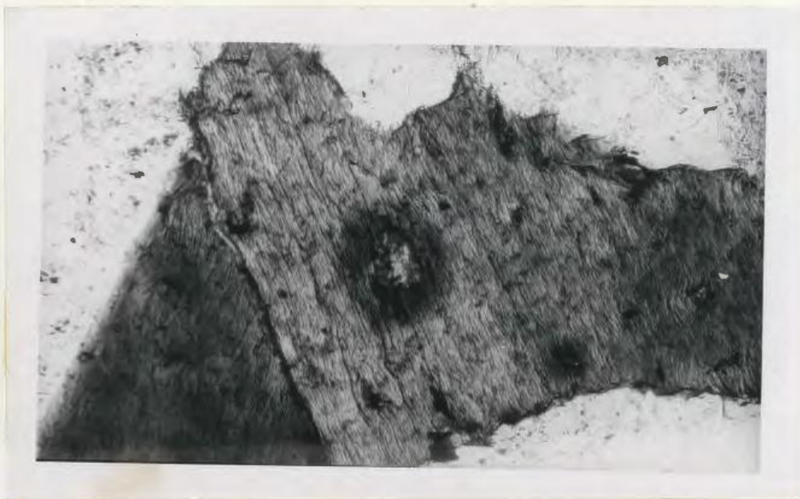
PLATE II-5: (X63, plane polarized light). Pleochroic halo around apatite inclusion in biotite.
