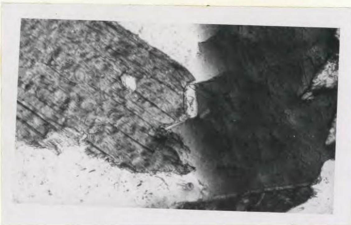
PLATE II-3: (X63, plane polarized light). Zircon inclusions in biotite.
