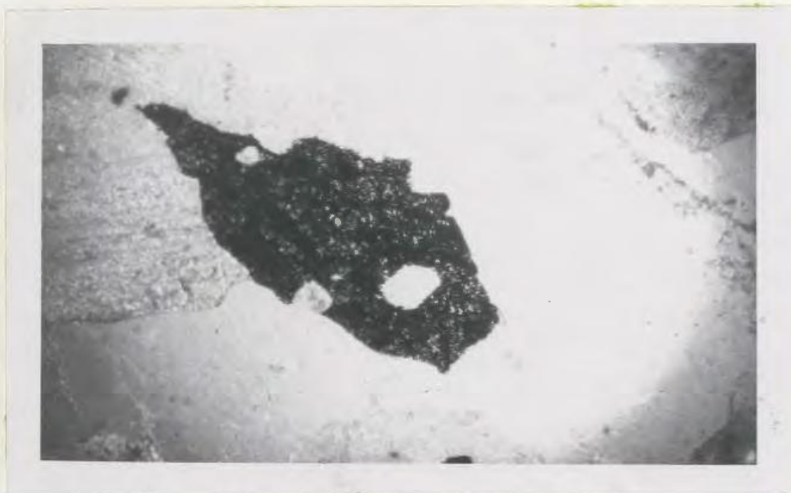
PLATE II-6: (X10, plane polarized light). Sphene crystal showing angular rhombic cross section.
