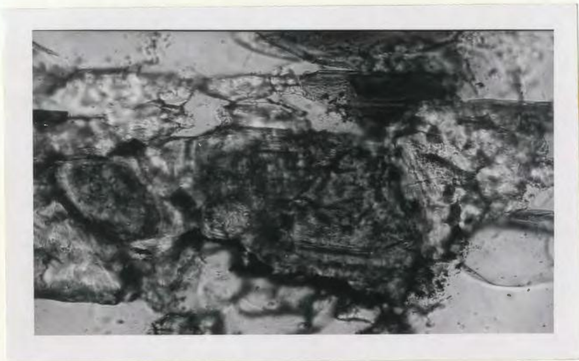
PLATE II-1: (X160, plane polarized light). Allanite crystal (dark grey) surrounded by rim of epidote (light grey).
