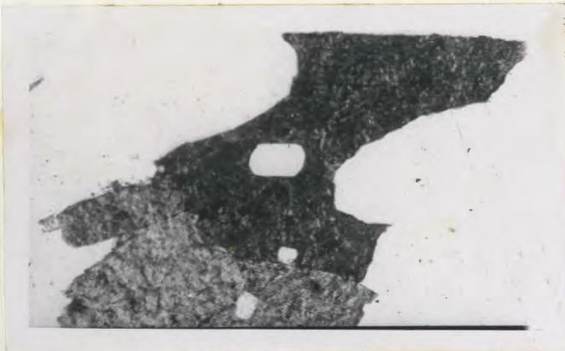
PLATE II-2: (X40, plane polarized light). Apatite inclusions (small white crystals) in biotite.
