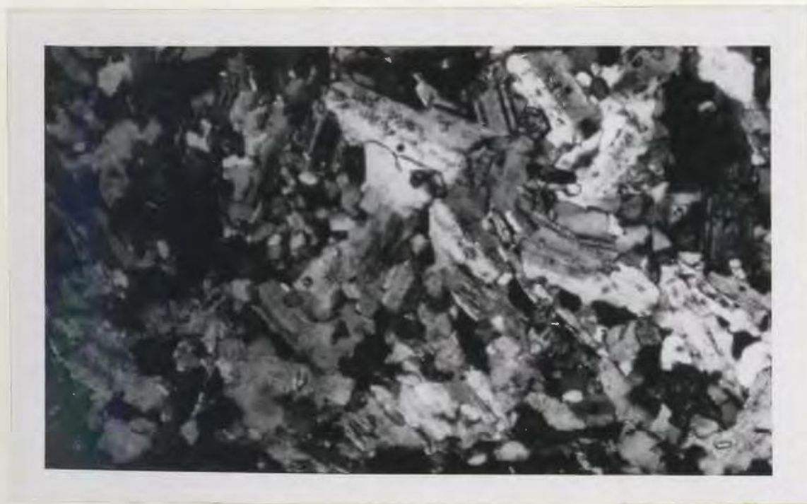
PLATE II-8: (X10, X nicols). Original igneous texture in altered diabase dyke.
