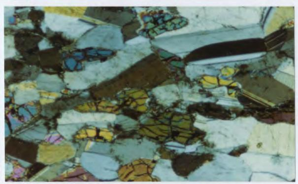
Figure 4.4. Troctolite with oriented elongate anhedral olivine with plagioclase. 79HPAD263-4. Crossed polars. 2 mm.
