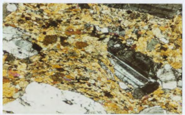
Figure 4.10. Amphibolite composed of near equal amounts of hornblende and plagioclase, and relict primary plagioclase grains which deflect the foliation. 78HPAD202-3. Crossed polars. 2 mm.
