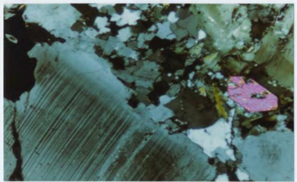
Figure 4.11. Trondhjemite, coarse grained with coarse hornblende (pale green - upper right) and strongly zoned plagioclase, both with ragged margins in groundmass of fine grained anhedral quartz and feldspar. Zircon is euhedral (pink) grain at right. 80HPAD223-1. Crossed polars. 2 mm.
