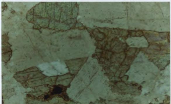
Figure 4.12. Trondhjemite, medium grained, composed of subhedral feldspar and primary epidote in an intersertal texture. Sample contains abundant oxide, rimmed by sphene. 79HPAD212-2. Plane polars. 2 mm.
