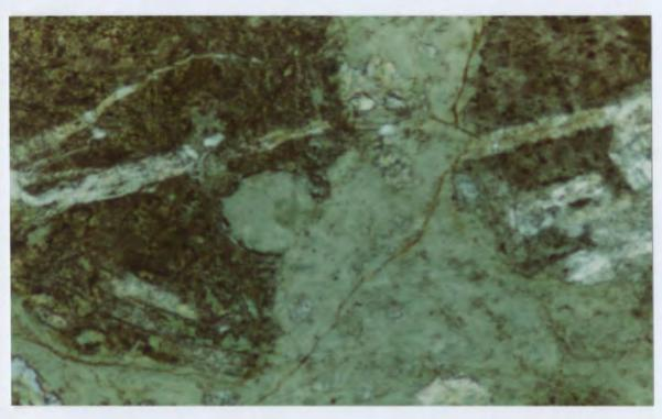
Figure 4.15. Brecciated dyke composed of angular to rounded fragments of fine grained, plagioclase porphyritic diabase (dark) in a matrix of chlorite + epidote (pale green). Spherical amygdules, this one broken into the matrix, also contain chlorite + epidote as does the veinlet cutting the fragment (upper right). 79HPAD200-1. Plane polars. 2 mm.
