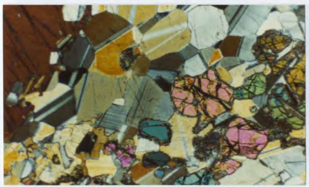
Figure 4.2. Olivine gabbro layer showing equant, subhedral cumulus olivine, cut by veins of serpentine + magnetite, plagioclase with smooth grain margins and triple junctions and oikocryst of Cr-diopside (brown - at left) enclosing small plagioclase grains. 79HPAD263-3. Crossed polars. Width= 4 mm.
