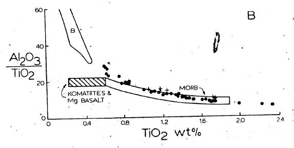
Figure 5.7A,B. CaO/TiO2 and Al203/TiO2 vs. TiO2 diagrams (after Sun and Nesbitt, 1978), for ophiolitic fragments. Explanation as for Figure 5.6. Analyses of dykes and pillow lavas plotted using the same symbols as Figure 5.2B. The majority of samples fall in the field of MORB.
