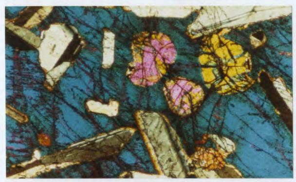
Figure 4.3. Troctolite sill with subhedral 'cumulus' olivine and plagioclase grains enclosed in a large Cr - diopside oikocryst (blue). 80HPAD133-5. Crossed polars. Width = 2 mm.
