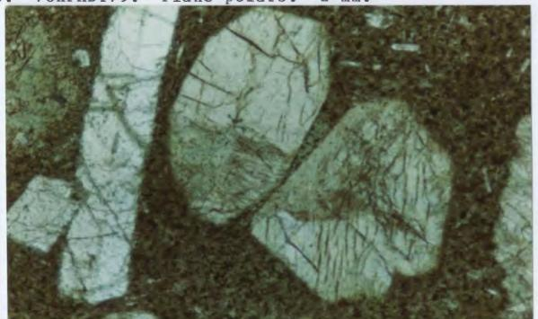
Figure 4.14. Same dyke as above with fine grained matrix and plagioclase and clinopyroxene phenocrysts. Clinopyroxene is partially altered to amphibole. 78HPAD179. Crossed polars. 2 mm.
