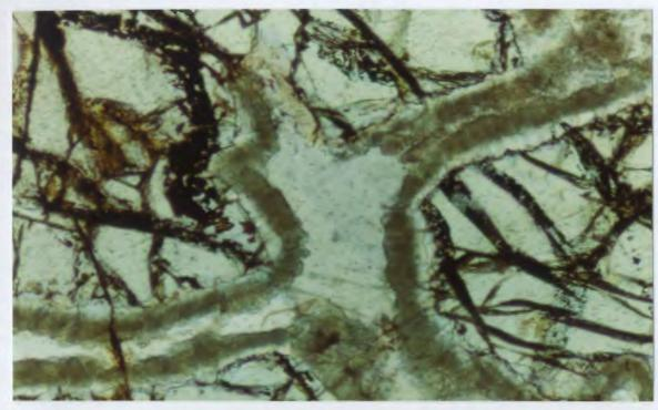
Figure 4.7. Corona texture in troctolite. Coronas separate olivine and plagioclase grains and show concentric zonation. 79HPAD269-3. Plane polars. 1 mm.
