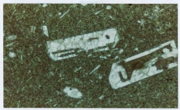
Figure 4.13. Diabase dyke with matrix of fine grained plagioclase laths and felted amphibole. Quenched plagioclase phenocrysts show skeletal 'belt buckle' outlines. 78HPAD179. Plane polars. 2 mm.
