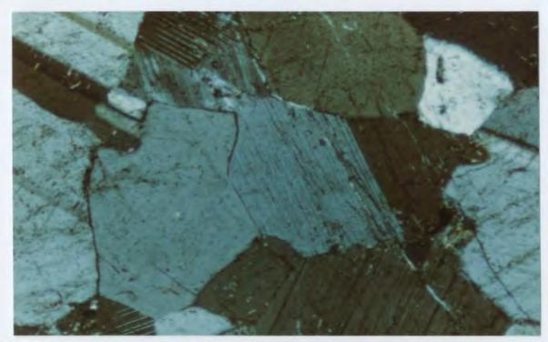
Figure 4.5. Anorthosite with coarse to medium grained plagioclase showing adcumulate texture with smooth grain boundaries and triple junctions. 79HPAD265-4. Plane polars. 2 mm.
