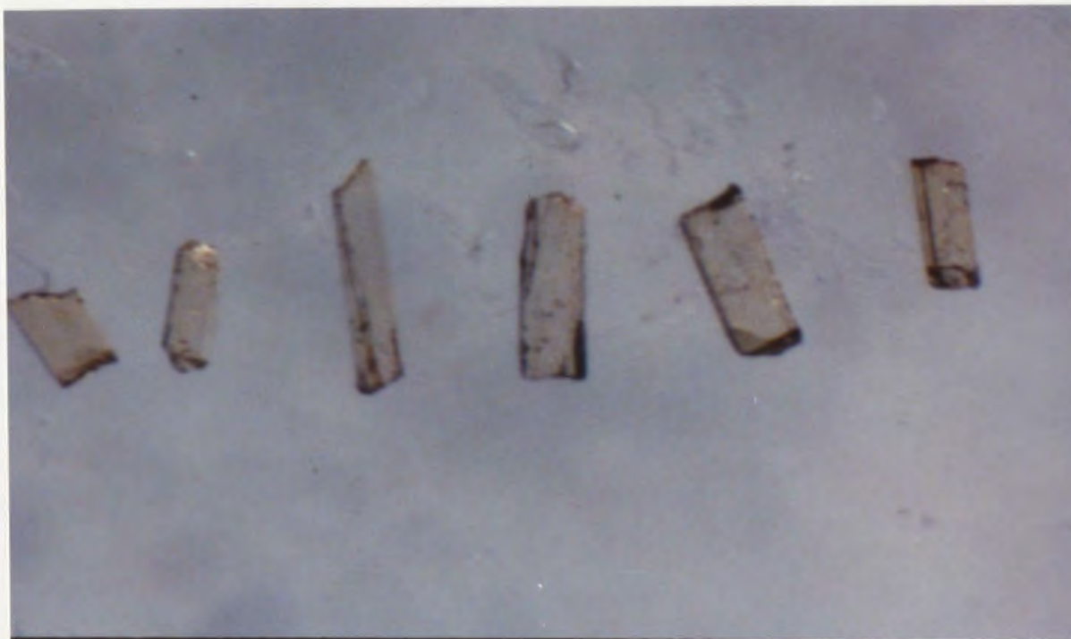
Plate 5.10. Small yellow-brown elongate zircon crystals in sample CSJ-10.
