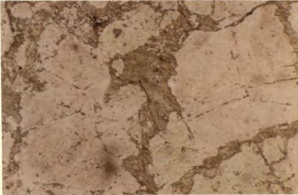
PLATE XIIa: Green biotite developed interstitially in quartz-diorites, Little Port Complex. Plain light x 90.
