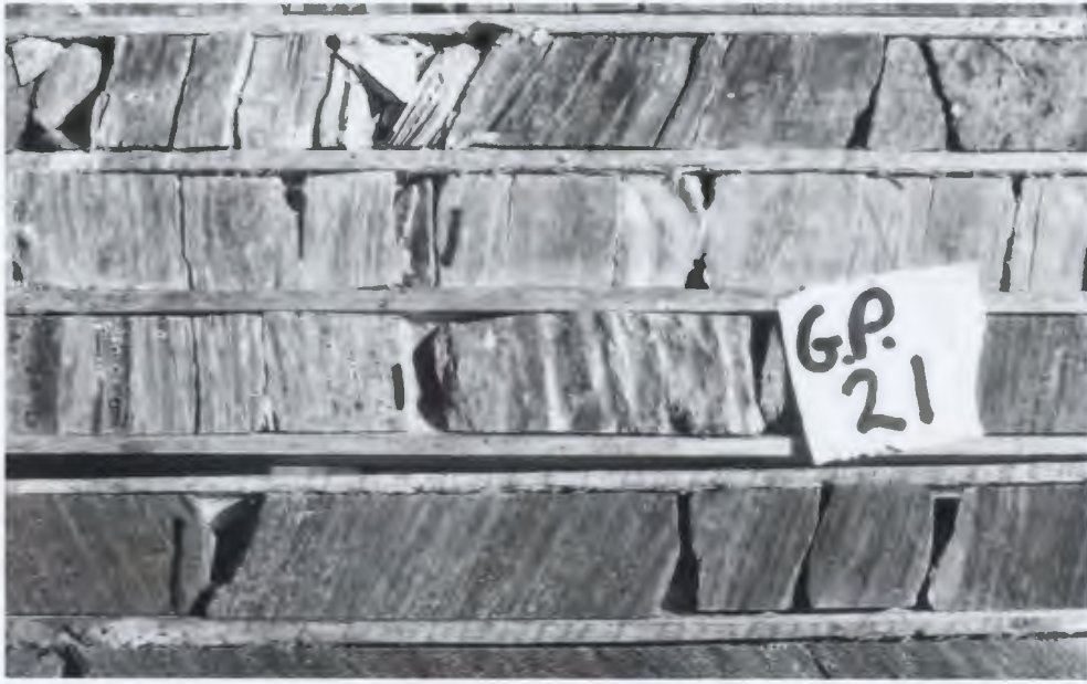
Plate 5.2 Rectangular brown patches of kaolinite with white powdery rims of pyrophyllite developed in pyrophyllite-paragonite schist (felsic volcanic rocks) from the structural hangingwall. Section is from diamond drill hole GP-21.
