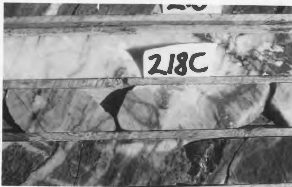
Plate 7.2 Close up of sample 218C showing dilational nature of veining and abundant stringers of fine-grained pyrite. This section assayed 7.3 g/t over 0.9 m.
