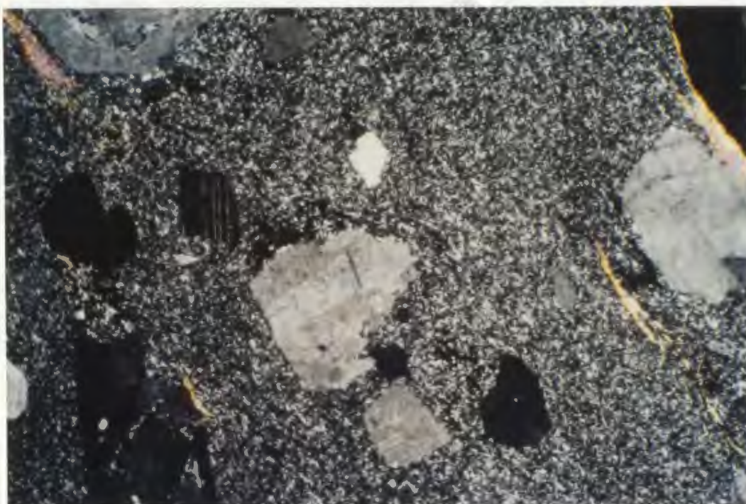
Plate 3.5 Photomicrograph of a weakly deformed felsic crystal tuff from Unit 3 (field of view is approximately 3.25 by 5 mm). Quartz and feldspar phenocrysts are developed in a quartzo-feldspathic matrix. The quartz phenocrysts exhibit undulatory extinction and the feldspar phenocrysts show typical albite twinning. Small wispy patches of sericite define the cleavage.
