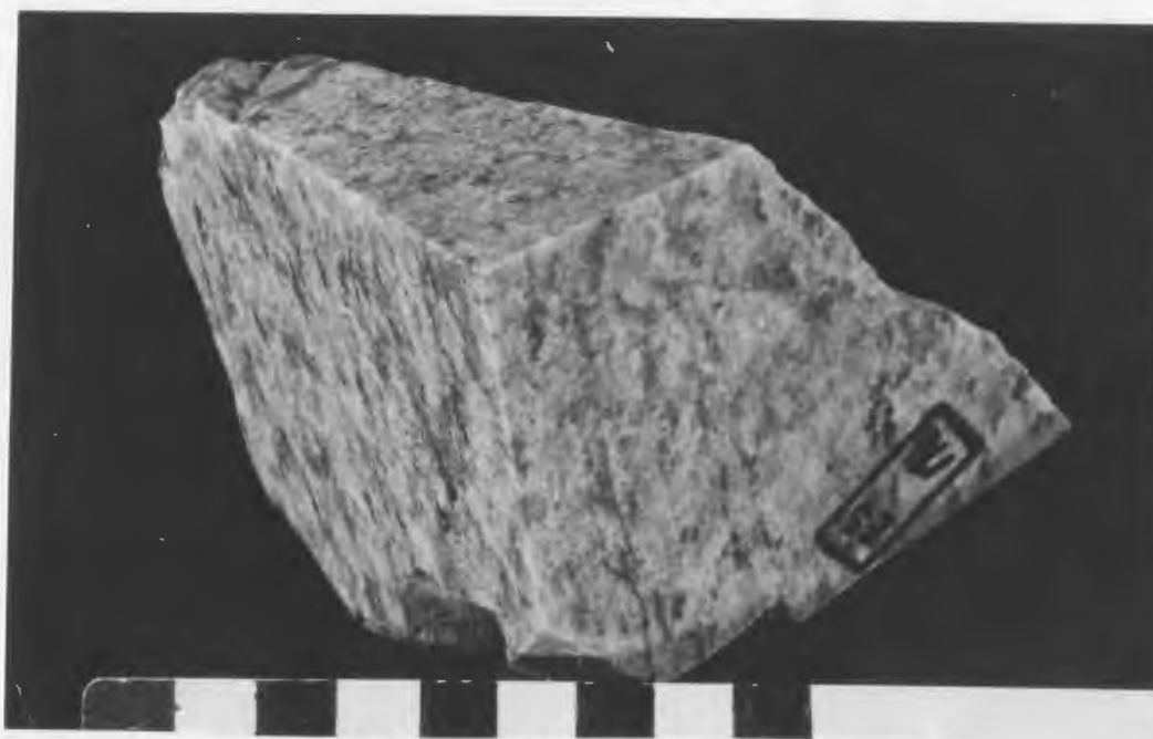
Figure 31: L 1 observed in the granite of South Trump Island. Here, L 1 is oriented vertically. Scale: 1 block = 1 cm.
