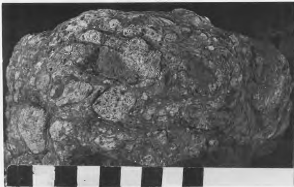
Figure 23: Hand specimen of diatrema material from the tip of Long Point, Twillingate. Scale: 1 block= 1cm.
