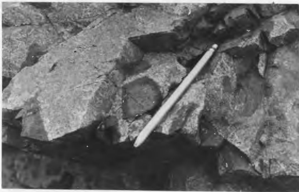
Figure 21: Close-up of the granite/basalt contact at Jenkins Cove. Note the absence of a chilled margin at this location.
