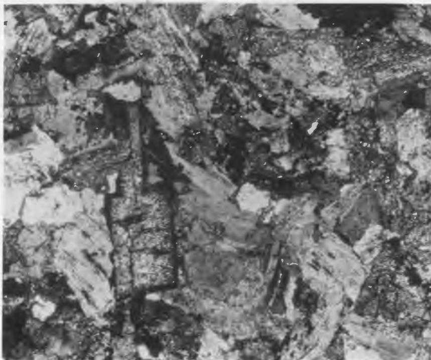
Figure 13: ES-1052. Diabase Dyke from the southeastern corner of Salt Harbour Island. X polars. The mineralogy of this dyke is identical to ES-1020. This is the dyke which was dated at 473 \pm 9 ma. by Williams et. al. (1976). Scale: 1cm=.25mm.
