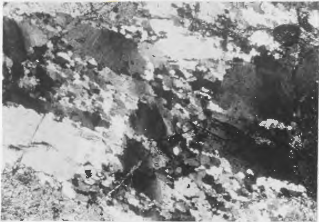
Figure 18: ES-1001. Deformed Granite from Gunning Head. X polars. Note the presence of small new grains at the boundaries of the larger, elongate quartz grains. Scale: 1cm=.25mm.
