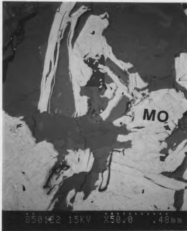
Figure 4-40: (850122) SEM back scatter image of fibrous molybdenite (MO-light grey) intergrown with quartz and feldspar in the leucocratic contact zone of the Burnt Lake Granite.
