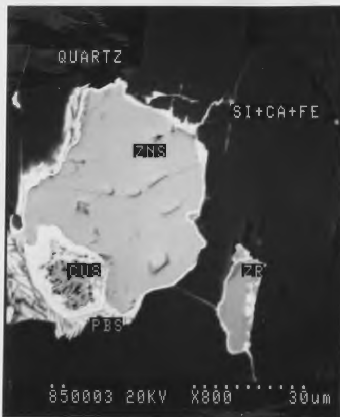
Figure 4-36: (850003) SEM back scatter image of an intergrowth of sphalerite (ZNS), chalcopyrite (CUS) and galena (PBS) in a quartz-plagioclase (SI+CA+FE) gangue. Note the small zircon (ZR) grain in the lower righthand corner.
