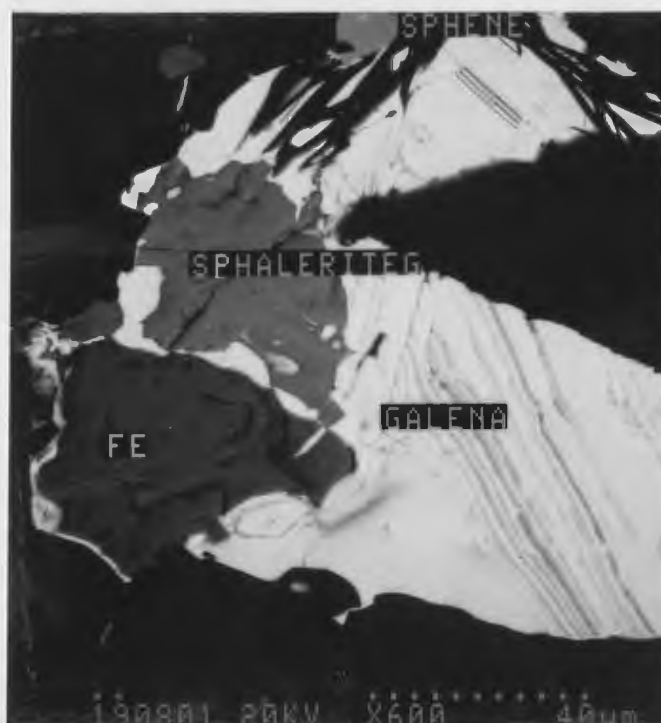
Figure 4-37: (190801) SEM back scatter image of intergrowth of galena, pyrite (FE), sphalerite and sphene in a Na-Ca-Mg-Fe-Si gangue matrix.
