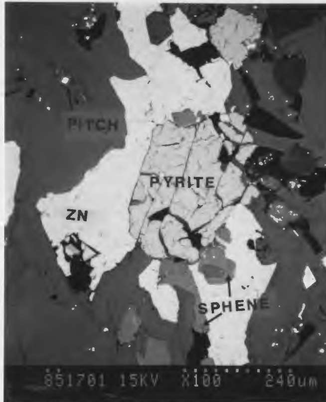
Figure 4-17: (851701) SEM back scatter image of sphalerite (ZN) intergrown with pyrite and sphene in a silicate gangue matrix (Si+Al+Mg). Small bright grains at the top of the photograph are uraninite (PITCH).
