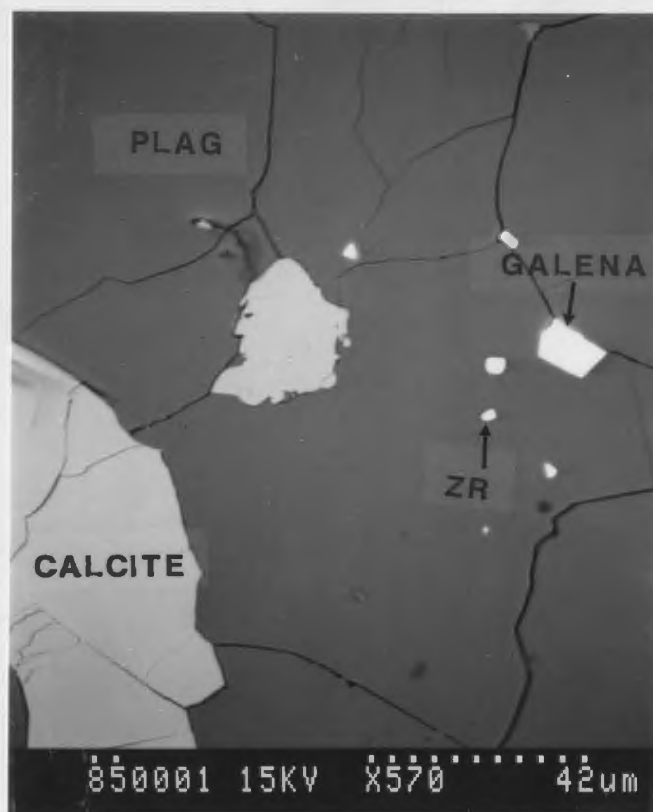
Figure 4-29: (850001) SEM back scatter image of euhedral galena and zircon (ZR) grains (white) in an interlocking mosaic of plagioclase (dark grey). A calcite veinlet occurs in the lower left corner of the photo (light grey).
