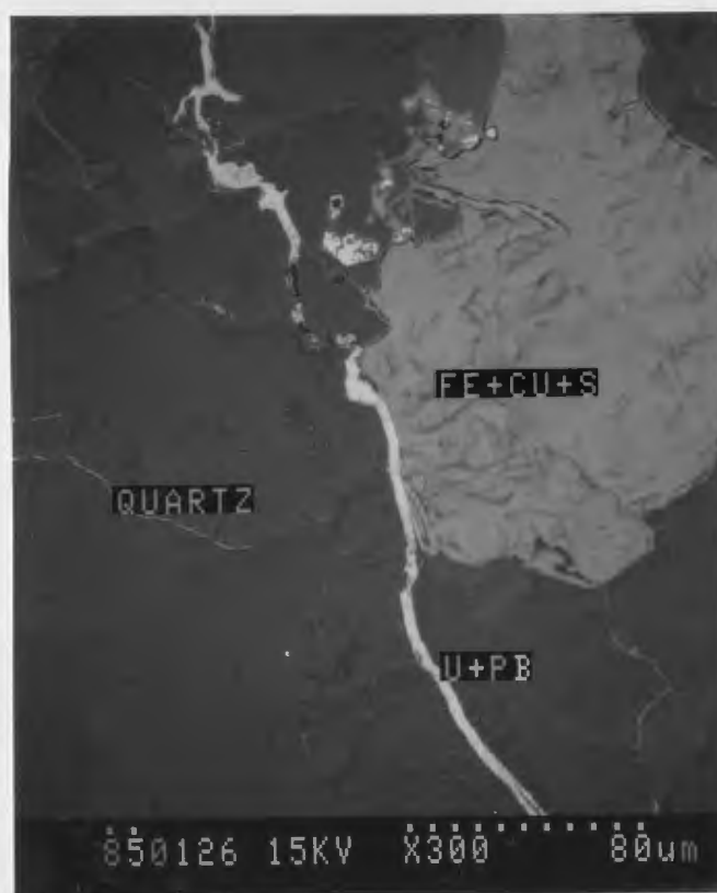
Figure 4-8: (850126) SEM back scatter image of chalcopyrite (FE+CU+S) intergrown with quartz (QUARTZ) gangue matrix and a uraninite (U+PB) veinlet (white).
