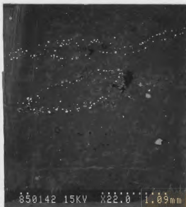
Figure 4-9: (850142) SEM back scatter image of magnetite (small white grains) rimming recrystallized feldspar porphyroblasts in a non-mineralized quartz-feldspar porphyry unit.
