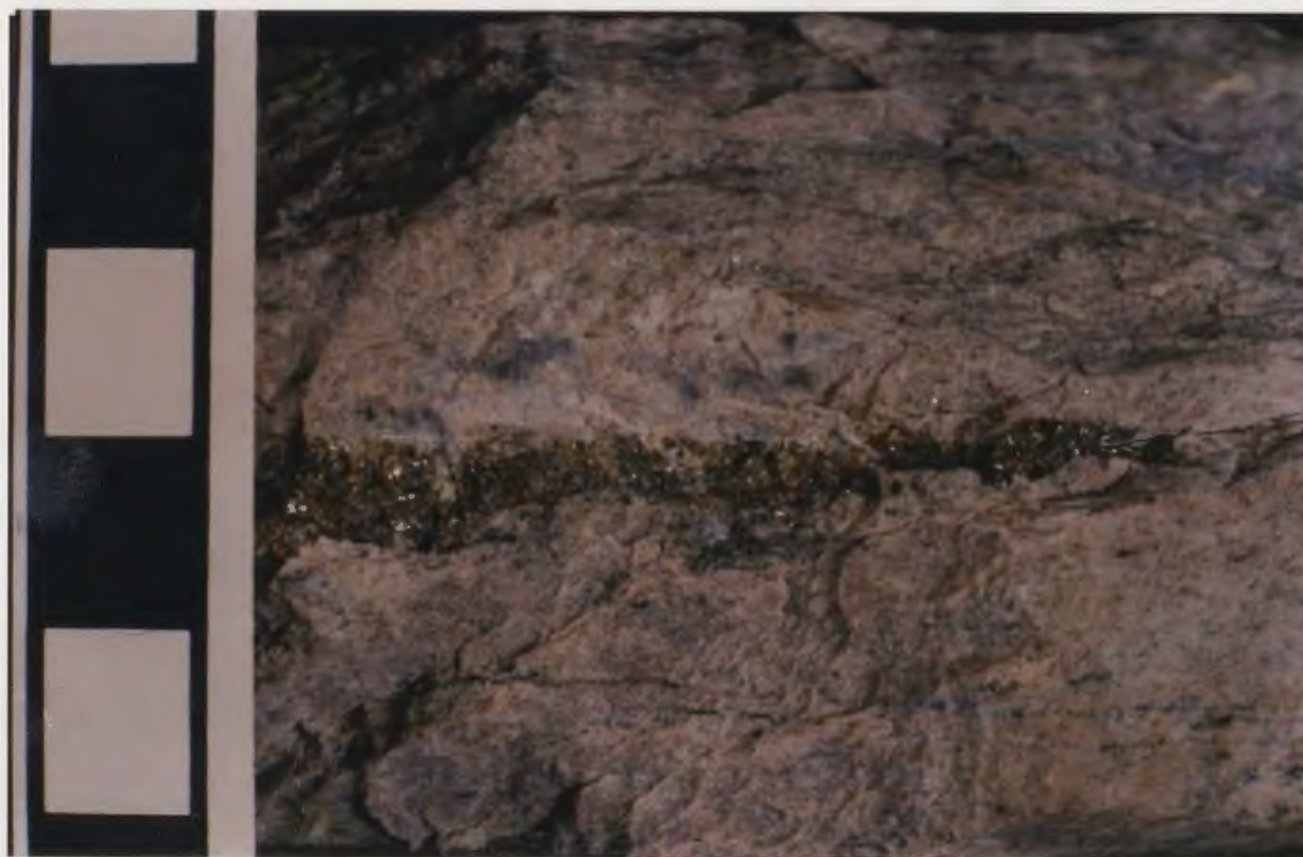
Figure 4-32: Recrystallized felsic tuff with a narrow veinlet of sphalerite. Scale bar is in centimetres.
