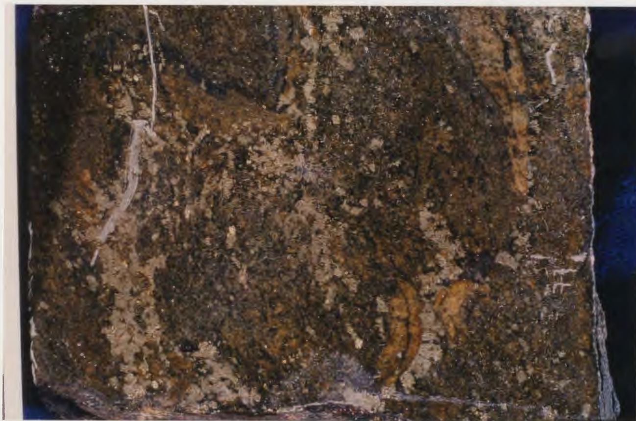
Figure 4-35: A cut section through extensive sulphide mineralization hosted by an altered mafic dyke. Sample EMS86-TR6 assayed 2.0% Zn, 0.58% Pb, 0.10% Cu, 0.43% U, 0.14% Mo and 22 ppm Ag. Note the tight fold in the lower righthand corner.
