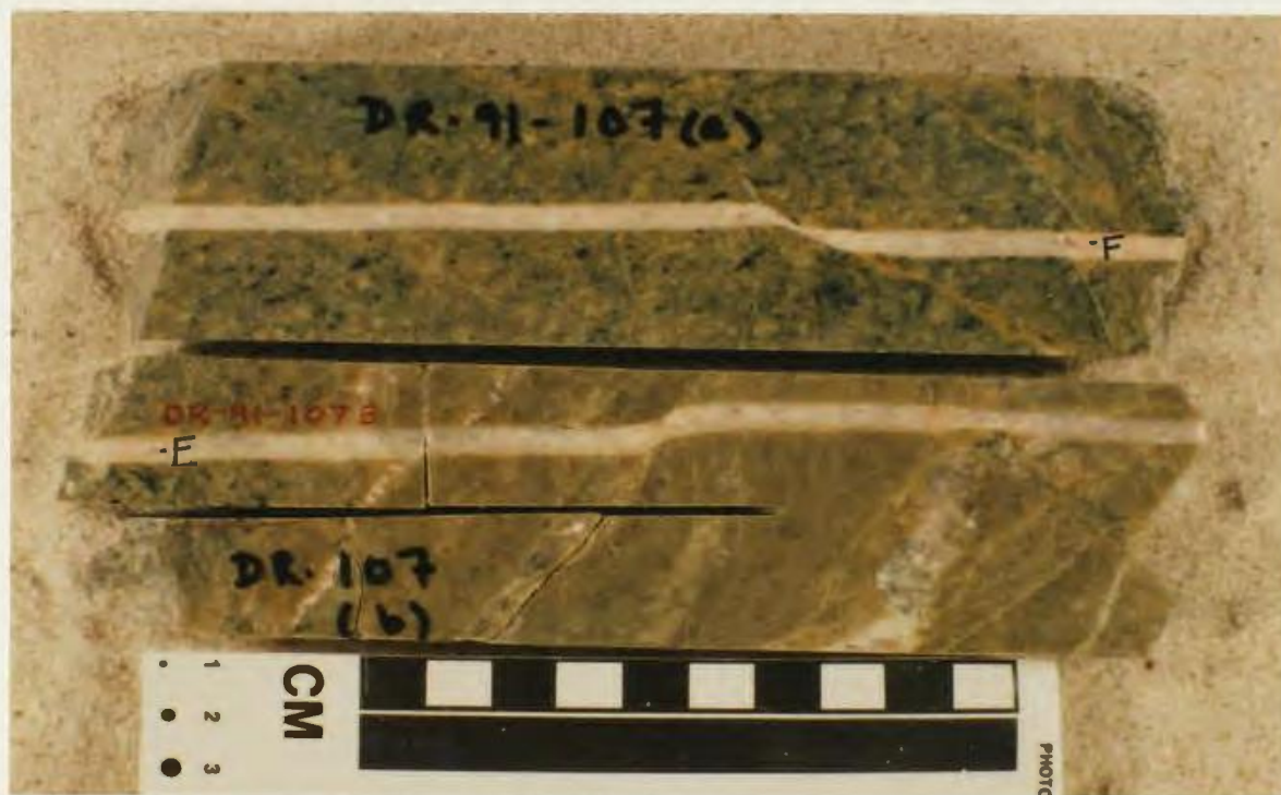
Plate 4.11 Fluorite (F, purple) in type III vein cutting S_2 fabric, but locally offset. Sample DR-91-107.
