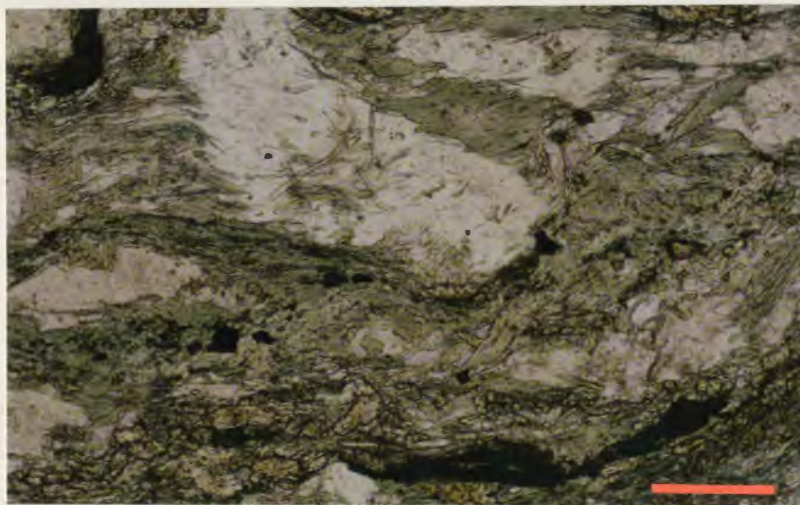
Plate 3.6 Epidote (high relief, yellow-brown), chlorite (green, patchy), and actinolite (bright green, acicular ) in metamorphosed basaltic rock, sample DR-90-28. View under crossed polars. Scale bar = 0.1 mm.
