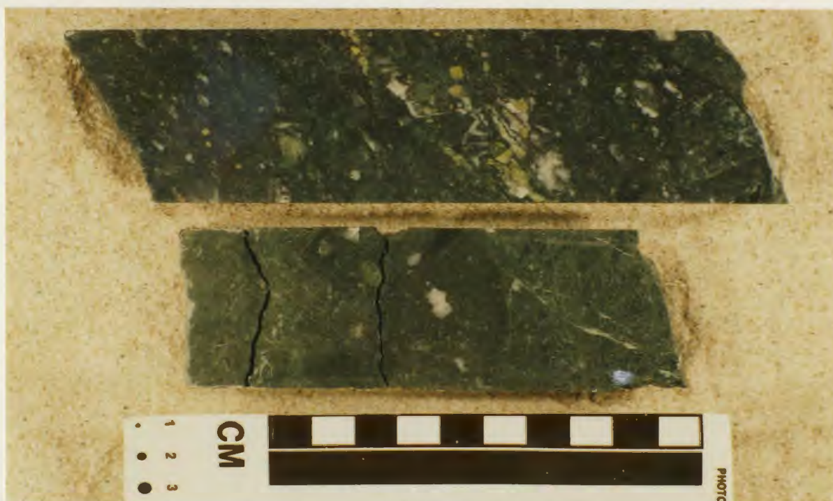
Plate 3.4 Unfoliated breccia of lower brittle fault in drill core DDH MS-89-27. Upper sample with abundant pale green epidote clasts is from 242 m depth, and lower sample with calcite veinlets and quartz fragments is from 243 m depth.
