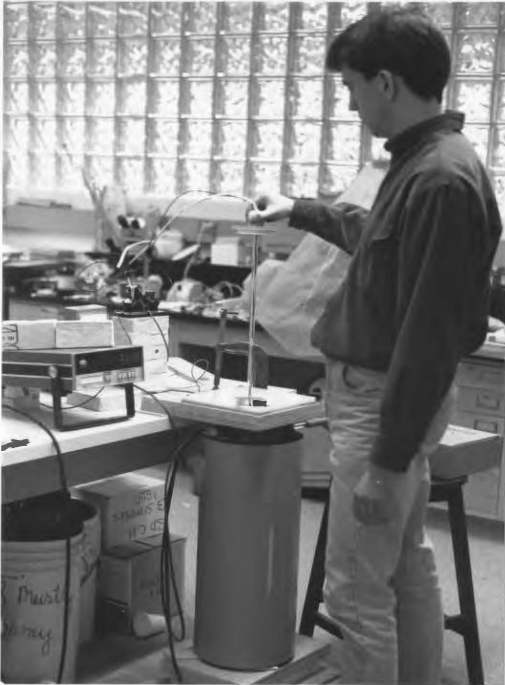
Figure 3.4: Photo of the dial and pyrex shaft being inserted in the specimen port.
