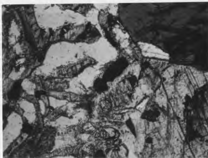
Fig. 4.3.3 B: Photomicrograph showing orthopyroxene relicts (in center) partly replaced by cummingtonite and with an outer rim of green amphibole. Clinopyroxene (bottom right) has a very narrow outer rim of amphibole. Sample: F84-84, PPL. Long dimension of figures corresponds to 0.75 mm.
