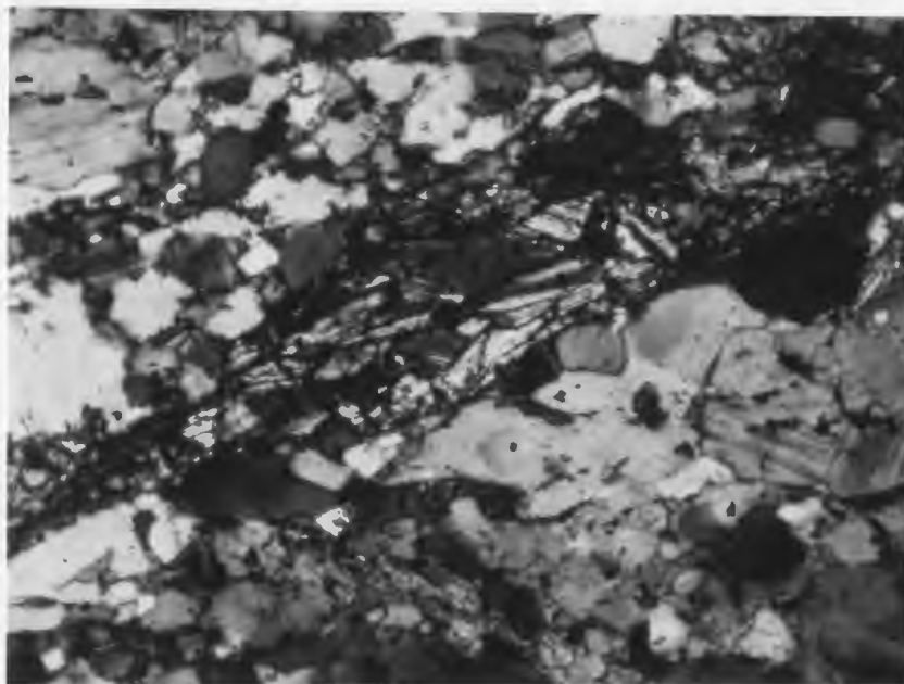
Fig. 4.3.3 A: Photomicrograph showing cummingtonite aggregate (center) after orthopyroxene. Sample: MZ-185a, XNic. Long dimension of figure corresponds to 0.75 mm.
