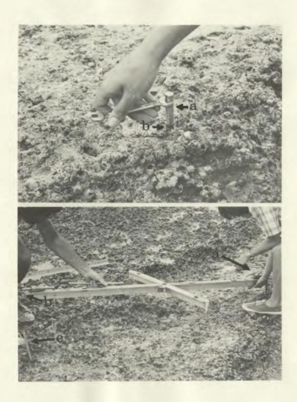
Plate 3. Rough levelling of the short axis of the bar is accomplished by locking the bar in position on the support pins (a) which slide into locking collars on the end of each short bar axis.
