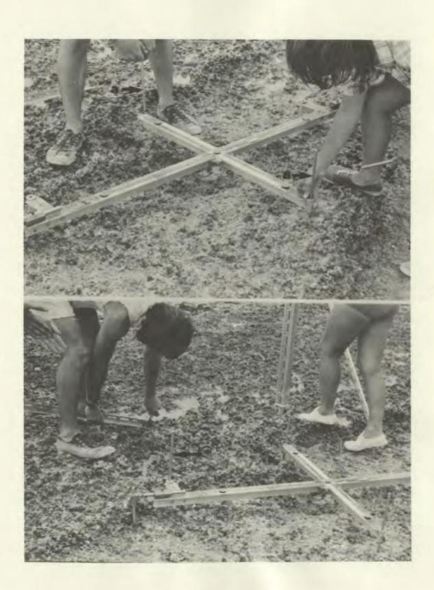
Plate 5. Upright dexion bars (a) are placed over the large pins and angle braces (b) are attached.
