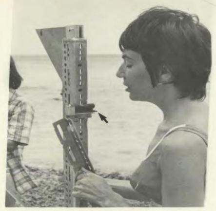
Plate 7. The horizontal camera bar is mounted on the uprights and bolted to the aluminum fins at the top of the uprights.
