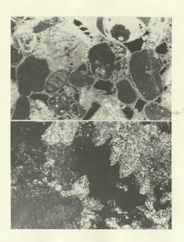
Plate 79. Thin section photomicrograph of rock from Section 47, Six Men's Bay, showing anhedral infilling of pore space by calcite. Note smaller dogtooth crystals perpendicular to the grain surface. Plane polarized light, 480x.
