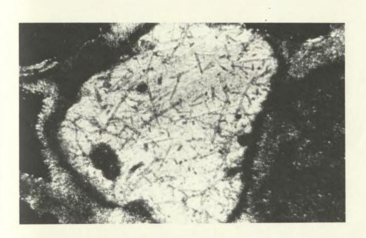
Plate 25. Scanning electron photomicrograph of a fractured grain disclosing straightwalled, penetrative type of boring. 1000x.
