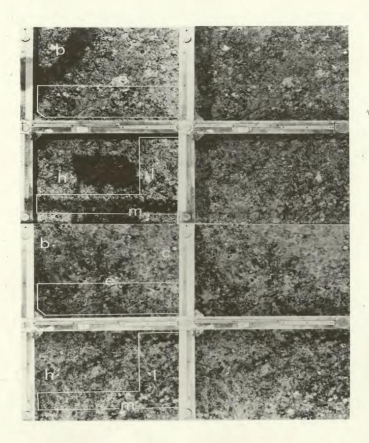
Plate 56. Photograph of right hand of Section (1973 photo). Areas outlined were analyzed photogrammetrically. Results were used to generate geomorphic zonal maps. Two distinct zones, shown in Overlay 1, were established:
