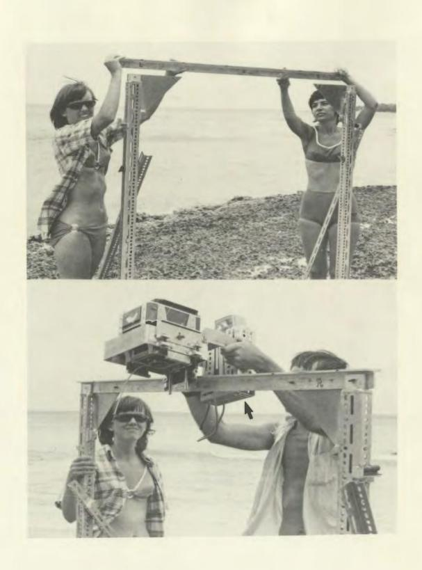
Plate 9. Five brass bezels (arrows) serve to define the zero datum reference plane from which all ground surface values are measured.
