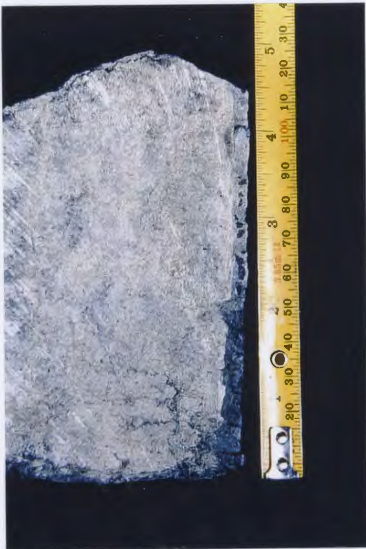
Figure 9o: Carbonaceous, loose shales of HF4 are frequently exposed as soil zones. Upper boundaries of HF4 shales are commonly truncated by coarse-grained sands ("soil zone", 3917.4 m, Hibernia C-96).
