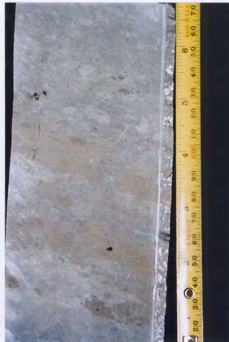
Figure 9l: Slightly-burrowed, churned, contorted and interstratified sandstone, siltstone and clayshales of HF2A. The lithology is encountered in association with coarser sandstone facies as the top member of fining-upward cycles (3,919.2 m, Hibernia C-96).
