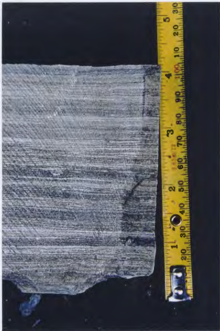
Figure 9i: Coarbonaceous and horizontally-laminated sands of HF1E1 also contain ripple cross lamination and lenticular sand beds (3,820.1 m, Hibernia K-18).
