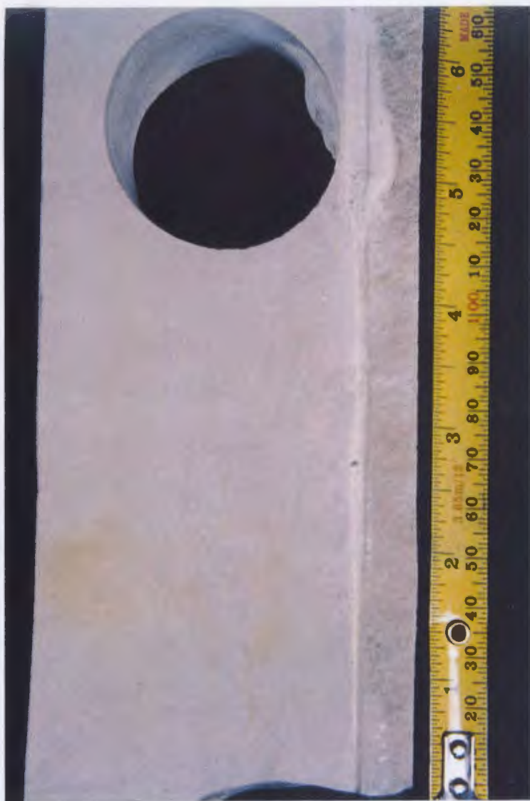
Figure 9a: Very fine-grained sands of HF1A are encountered with the fine-grained sands of HF1B in fining-upward sequences (3,797.25 m, Hibernia K-18).
