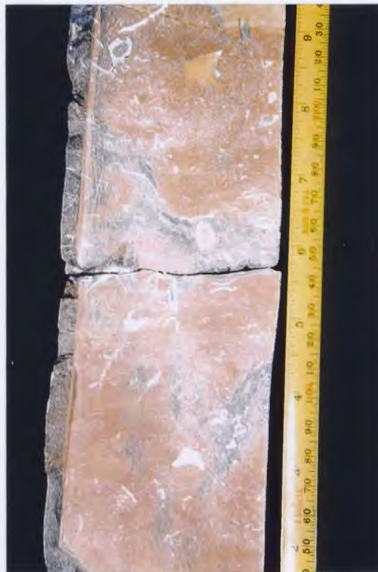
Figure 9p: Shales of HF5 contain shell fragments (3,950.8 m, Hibernia C-96).
