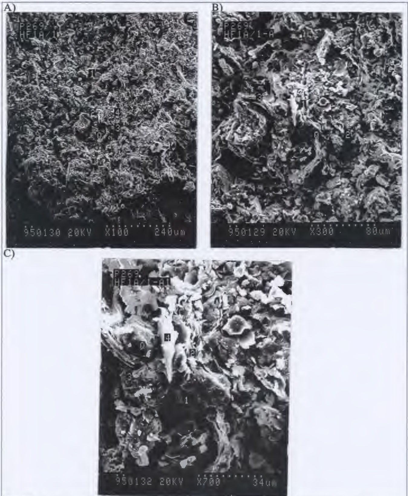
Figure 13: This specimen of HF1A is more argillaceous than SP102-HF1A. Elongated flaky minerals are muscovite. Siderite cement and smectite are the primary constituents as well as detrital quartz (Appendix 3).
