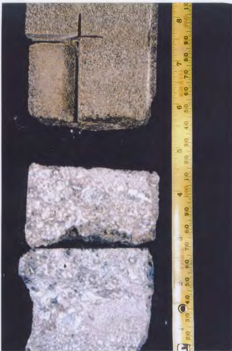
Figure 9g: Pebbly and bimodal sands of HF3 are basal lag sediments which form the base of fining-upward cycles. The photo shows the HF3 lithology in association with medium-grained sands (3,909.40m, Hibernia C-96).
