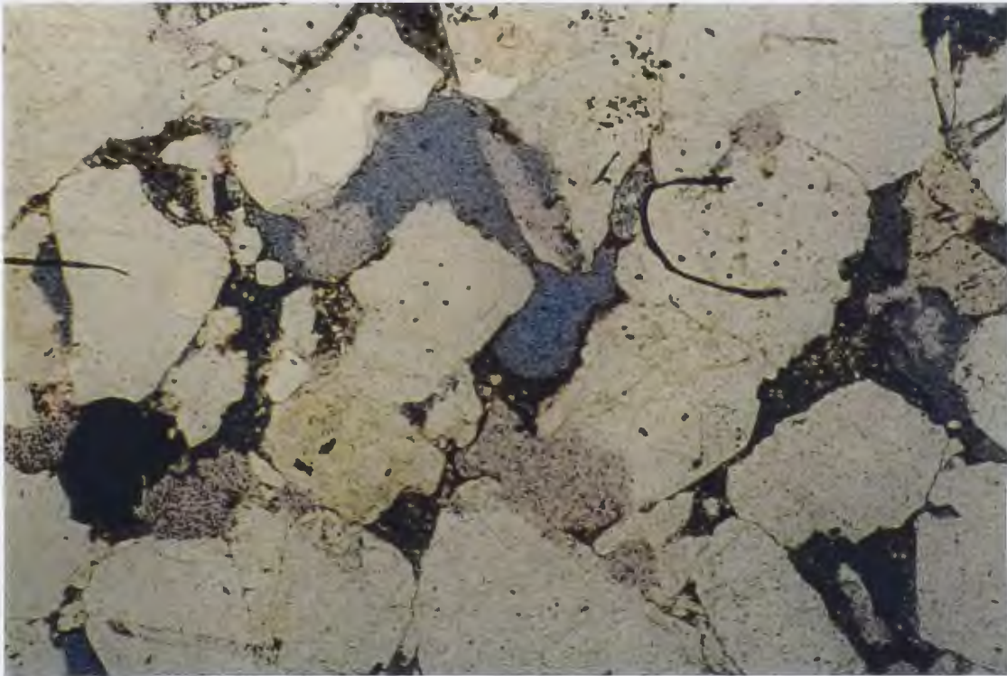
Figure 41b: HF1F . Preferential alignment of possible geopetal fill, good porosity and pore connectivity of the lithology can be observed in lower magnification photo. The lithology is subangular to subrounded, and moderately-sorted. (P74; Mag=X2PP) ( k=1290 mD; \phi = 19.3\% )
