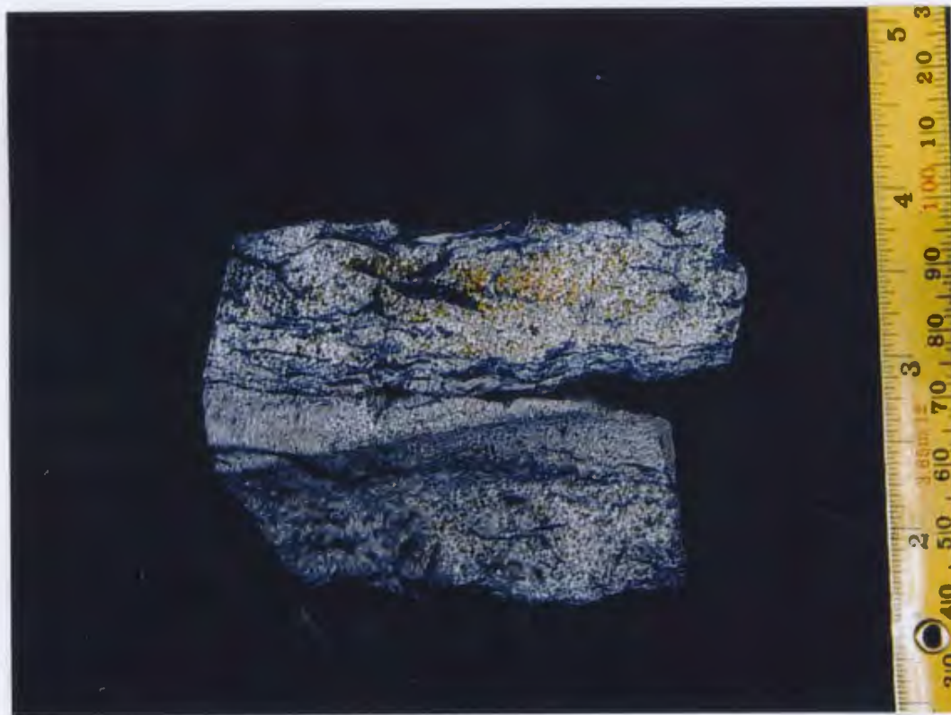
Figure 9k: Very carbonaceous, poorly-consolidated fine-grained sands of HF6 are also recorded only in Hibernia B-27 (3,848.4 m).
