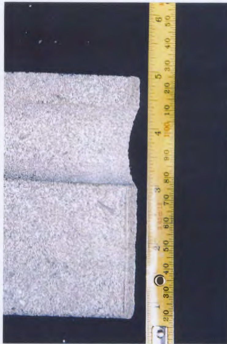
Figure 9f: Quartzitic basal sandstones of HF1F are coarse-grained. No evident structure other than a few faint crossbeds is observed in the lithology. HF1F sands are found in the bases of fining-upward cycles (3,923.2 m, Hibernia C-96).
