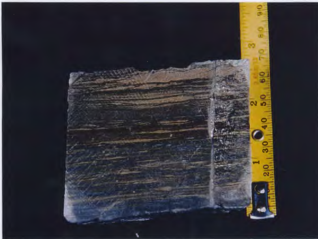
Figure 9m: High shale content and lenticular sand lenses are characteristics of HF2B (3,624.9 m, Hibernia B-O8).
