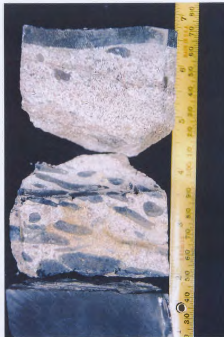
Figure 9d: Elongate rip-up mud clasts are abundant in the lower medium-grained sandstones of HF1C1 (3,939.50 m, Hibernia C-96).
