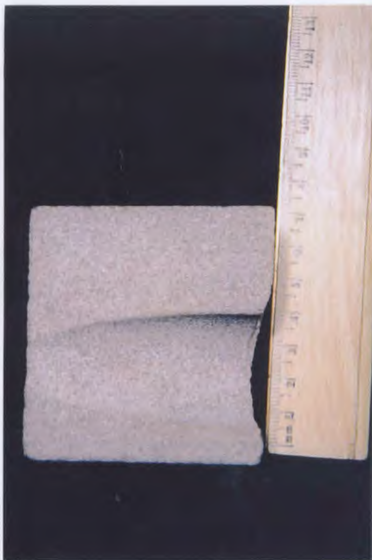
Figure 9c: Oil-wetted, upper fine- to lower medium-grained reservoir sands of HF1C constitute the main pay in the formation (3,935.70 m, Hibernia K-14).
