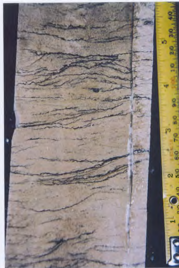
Figure 9h: Ripple cross lamination and abundant carbonaceous zones are evident in the very fine- to fine-grained sandstones of HF1E (3,622.18 m, Hibernia K-18).
