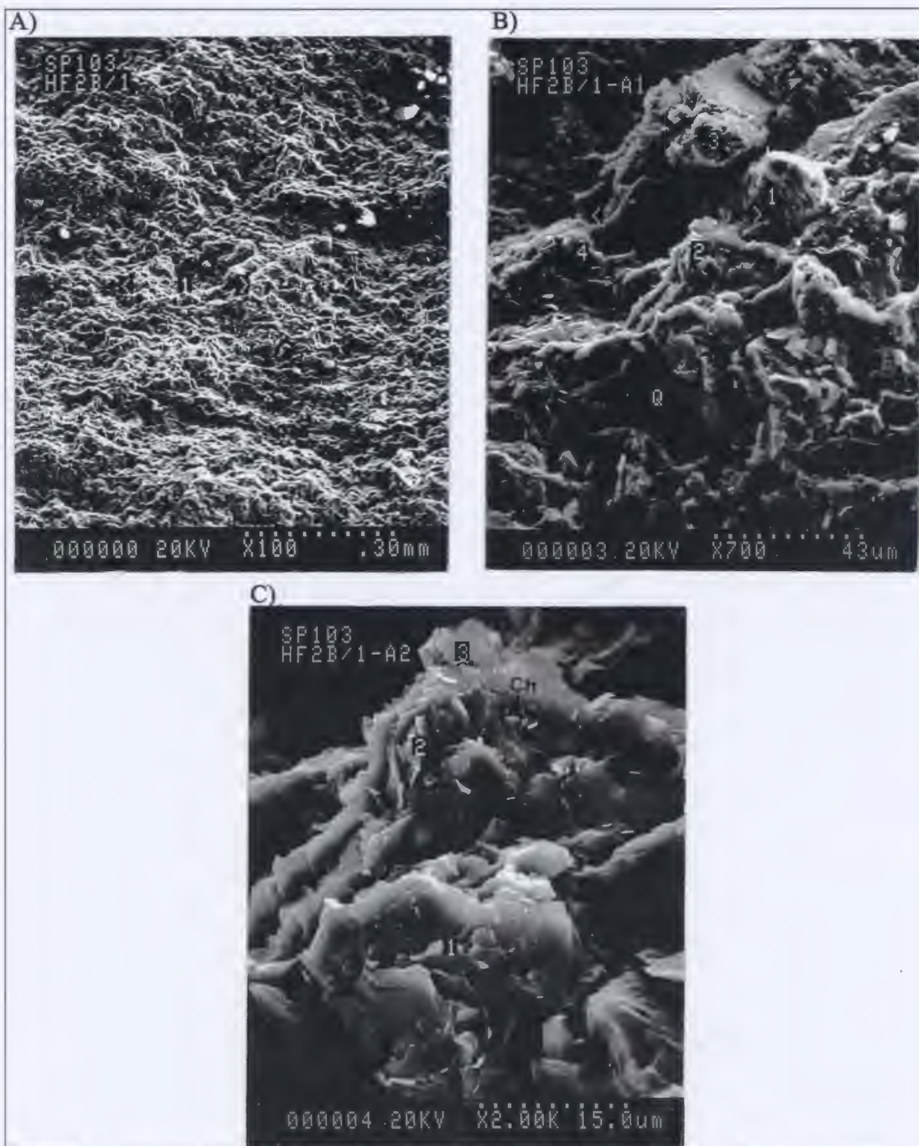
Figure 34: SP103-HF2B is more argillaceous than HF2A specimen. Clay- and mica-rich character of the specimen yielded very complex elements detections in the SSQ analysis. Kaolinite is identified at point "3" and "4" in 34b . X2,000 mag. helped to visually identify chlorite (Ch) in the argillaceous clusters (Kaolinite="3" in 34b, Muscovite="1" in 34c, Ch=Chlorite)(Appendix 3).
