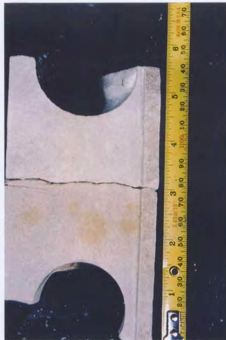
Figure 9b: Well-consolidated, fine-grained quartz sandstones of HF1B are slightly oil-stained (3,807.50 m, Hibernia K-18).
