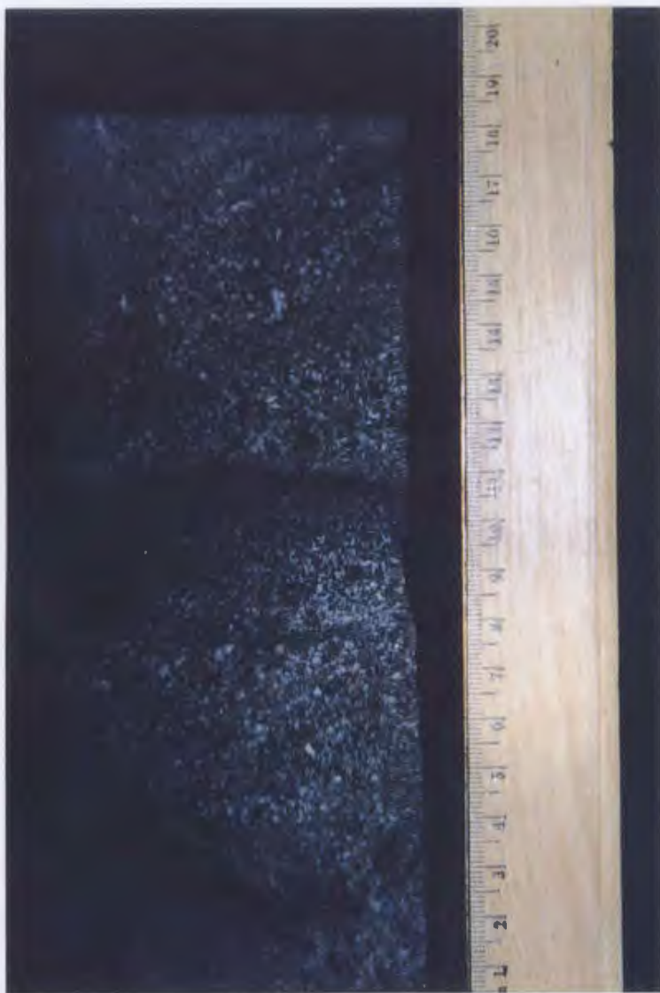
Figure 9e: Carbonaceous, quartzitic, medium- to coarse-grained sands of HF1D. Sedimentary structures are not preserved (3,869.70 m, Hibernia K-14).
