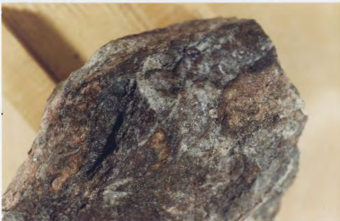
Plate 3.12. LPW-type vein mineralization from Long Pond West #1 showing. Note the quartz-fuchsite vein material cross cutting the earlier quartz-dolomite alteration assemblage (red-brown).
