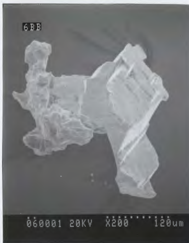
Plate 3.13. Scanning electron micrograph of detrital gold grain from overburden above LPW-type vein. Negative carbonate crystal imprint attests to an association between carbonate and gold in the vein.
