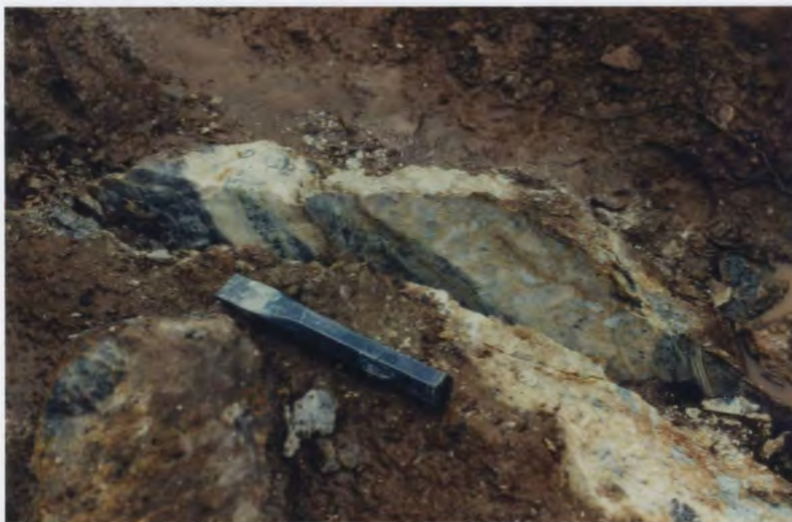
Plate 3.1. L-type vein mineralization. Tabular quartz (white) and magnesite (orange-brown) veins within talc-magnesite altered ultramafic rock (blue-grey).
