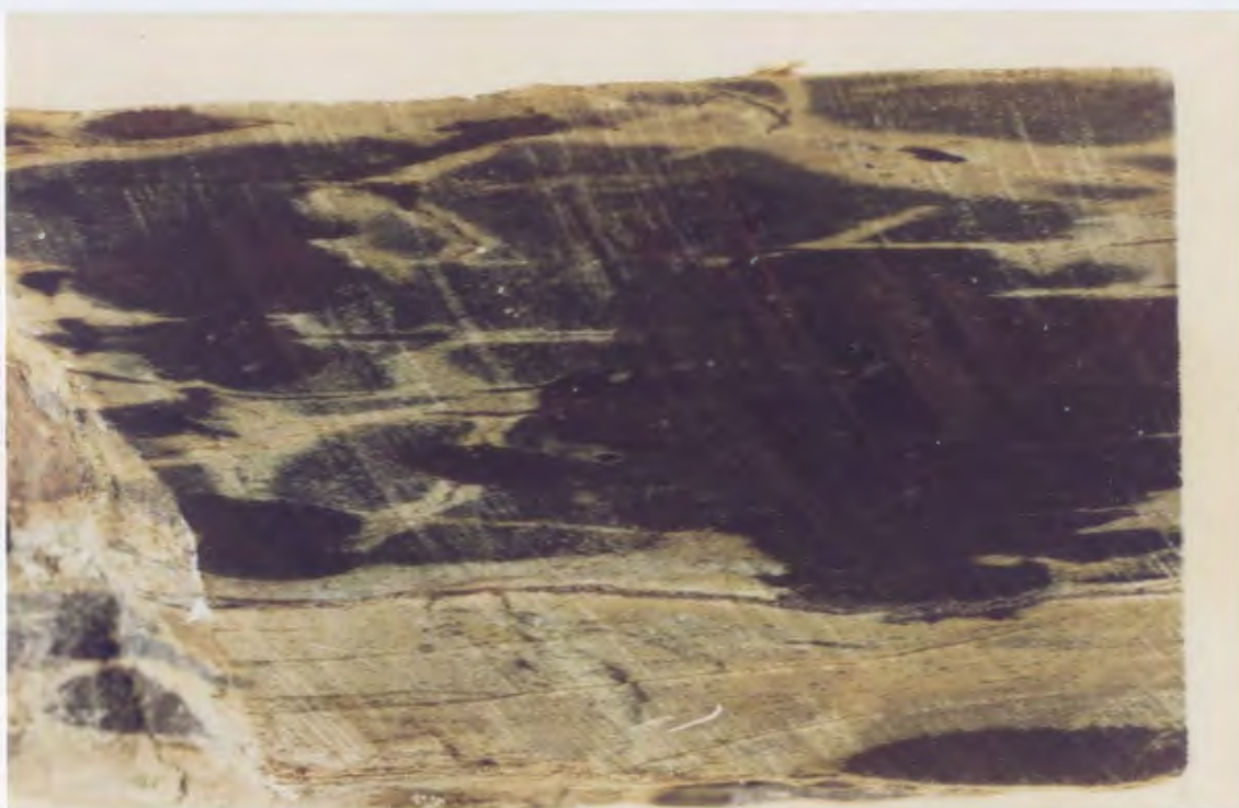
Plate 3.19. Pervasive alteration of mafic volcanic rock adjacent to LPW-type vein at Long Pond West. Bleaching (sericitization) is the first stage followed by hematization (dark purple) which overprints the sericitic alteration.
