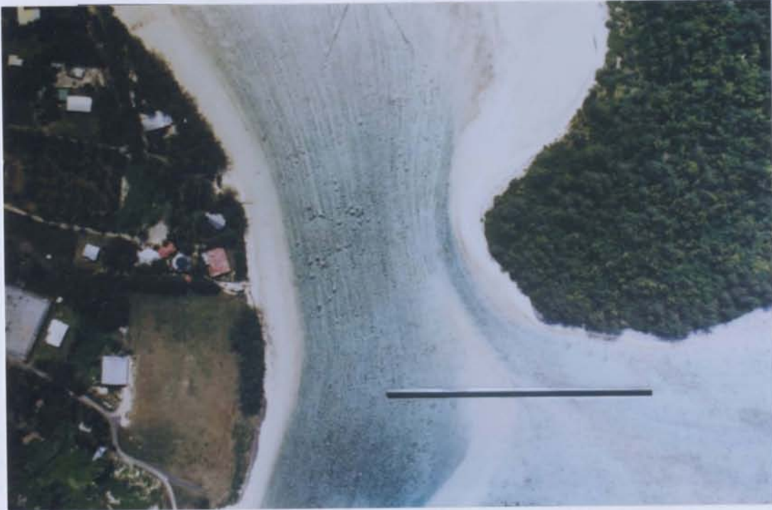
Plate 5.9 Aerial photograph of apparent striations in the channel between Oneroa and the mainland. They are formed as sand is deposited in the lee of large cobbles and boulders. Scale bar is 200 m.
