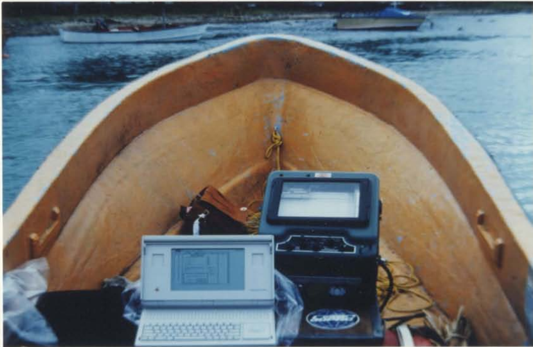
Plate 2.1 Echosounder attached to a portable computer in the bow of the small boat used to gather bathymetric data in from Ngatangiia Harbour.
