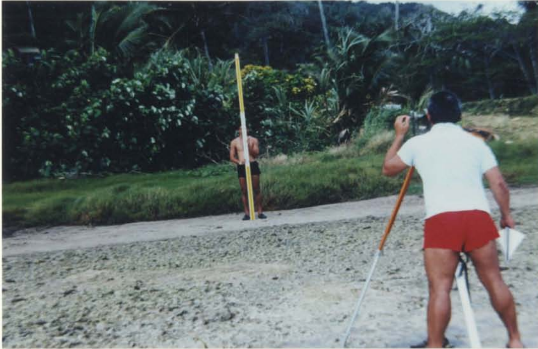
Plate 2.2 An example of the land-based compass and level survey technique used to record spot depths from the channel and lagoon.
