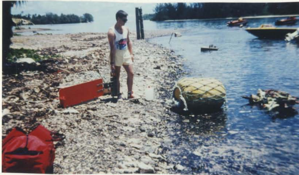
Plate 2.3 The current meter mooring placed at the entrance to Ngatangiia Harbour. The engine block anchor is at the far left centre; the float, enclosed in netting is at the water's edge and the author is holding the current metre.
