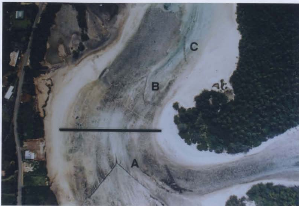
Plate 5.5 Aerial photograph of fish traps in the channel (A, B, C) showing associated accumulations of sediment (lighter areas at the apex of each trap). Scale bar is 200 m.
