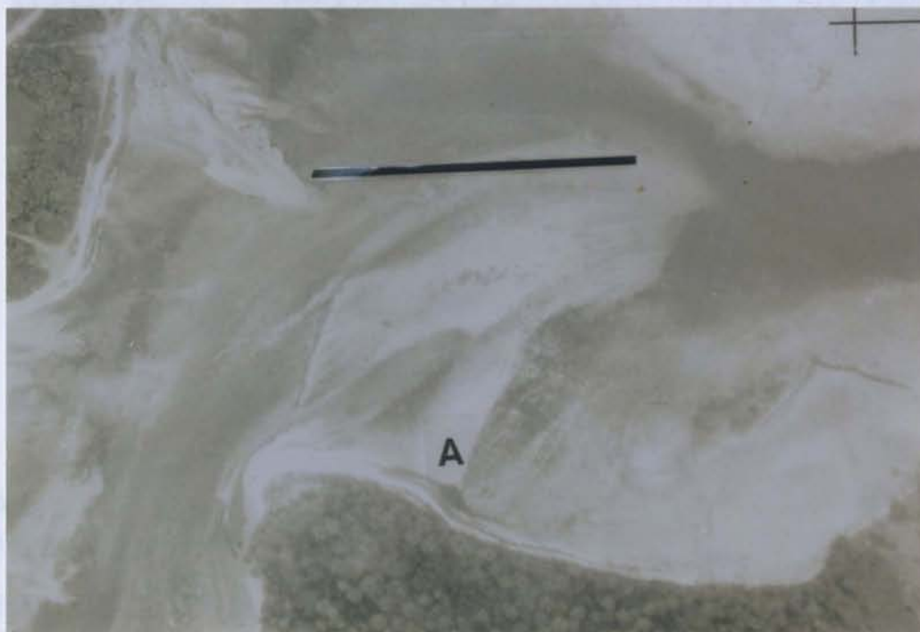
Plate 5.6 Aerial photograph of Ngatangia Harbour taken in 1954 showing the spit developed (A) at the northwest tip of Motu Tapu. North is to the top of the photo and the scale bar is 100 m.
