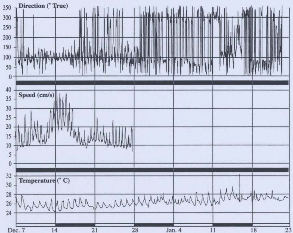
Figure 4.8 Current meter data from Ngatangia Harbour including salinity, temperature, E-W component of current, speed, and direction.
