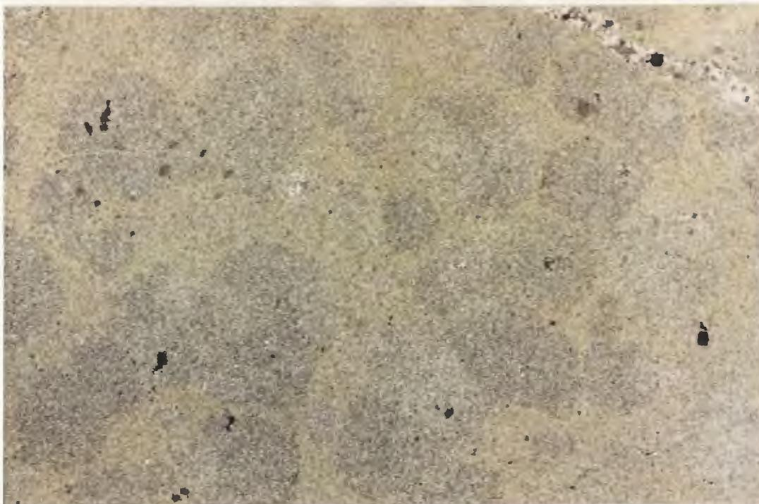
**Plate 2.7.** Relict spherulites composed of fine-grained quartz and feldspar in a matrix of fine-grained sericite and feldspar. Sample SS88-493 (584221), mag.= 7.5X, fov = 14.0 mm, X-nicols.
