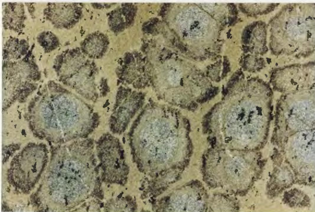
**Plate 2.8.** Relict spherulite containing fine-grained quartz-rich cores, inner sericitic mantles, and outer sericite-and opaque-rich mantles, in a very fine-grained sericite groundmass. Sample SS88-515, mag.= 8X, fov = 13.2 mm, X-nicols.
