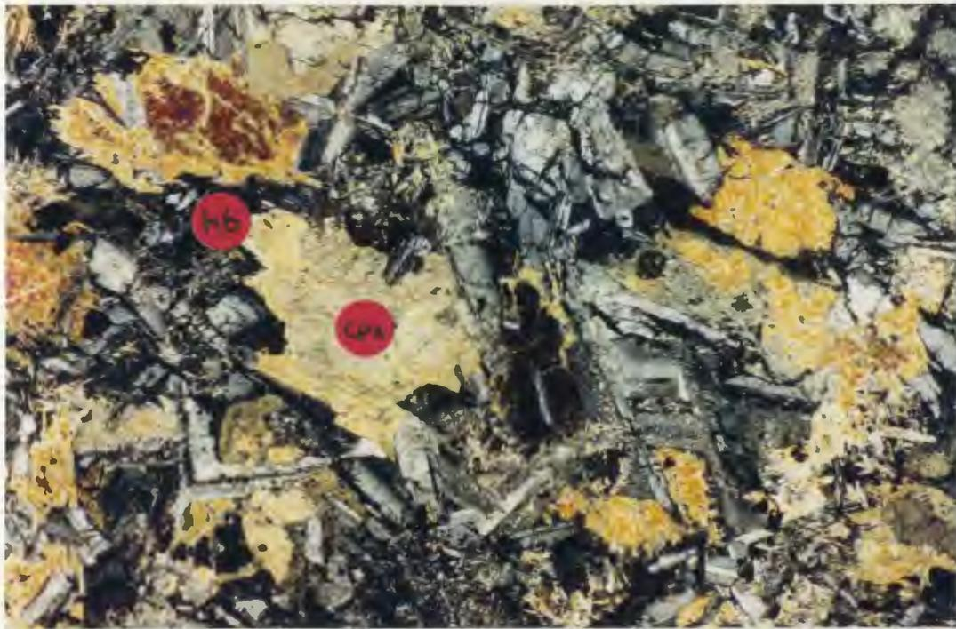
**Plate 2.13.** Hornblende (hb) replacing clinopyroxene (cpx) in a gabbroic phase of the Hermitage Bay Complex. Sample SS88-351 (584172), mag.= 20X, X-nicols.
