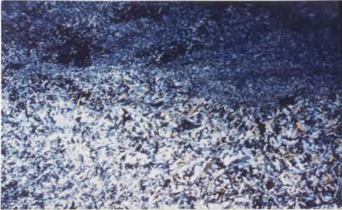
**Plate 4.17.** Layering in tremolite due to changes in crystal size. From the calc-silicate horizon (subunit 1g) at Winter Hill. Sample SS88-072 (584044), mag.= 20X, X-nicols.
