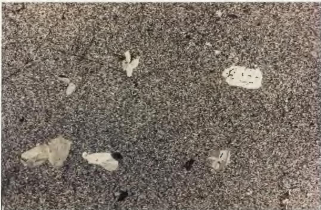
**Plate 2.14.** Older rhyolite dyke containing plagioclase phenocrysts in a fine-grained quartzo-feldspathic matrix. Sample SS88-062 (584034), mag.= 6.3X, fov = 17.0 mm, X-nicols.
