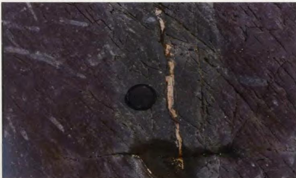
Figure 26. Vein BV5 in the town of St. Brides. Calcite has filled one fracture in a pre-existing fracture set. The sediments next to the vein have been altered from red to green, indicating the reducing nature of the source fluid.
