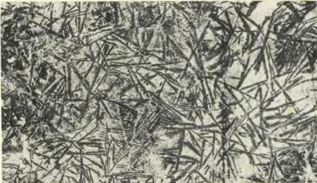
Figure 32: Photomicrograph of a pillow lava sample from near Betts Cove mine showing randomly oriented clinozoisite laths in a plagioclase-uralite groundmass. Plane polarized light (X15).
