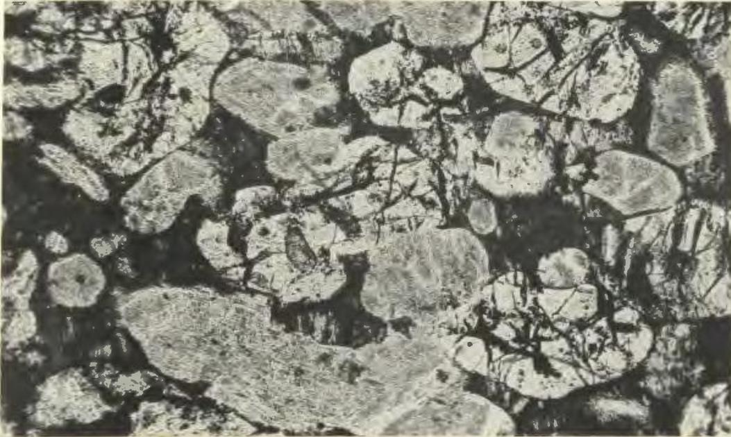
Figure 10: Photomicrograph showing cumulate serpentized olivine (with black magnetite-bearing veins) and talcose orthopyroxene (grey) surrounded by intercumulate clinopyroxene (black). Plane polarized light (X40).
