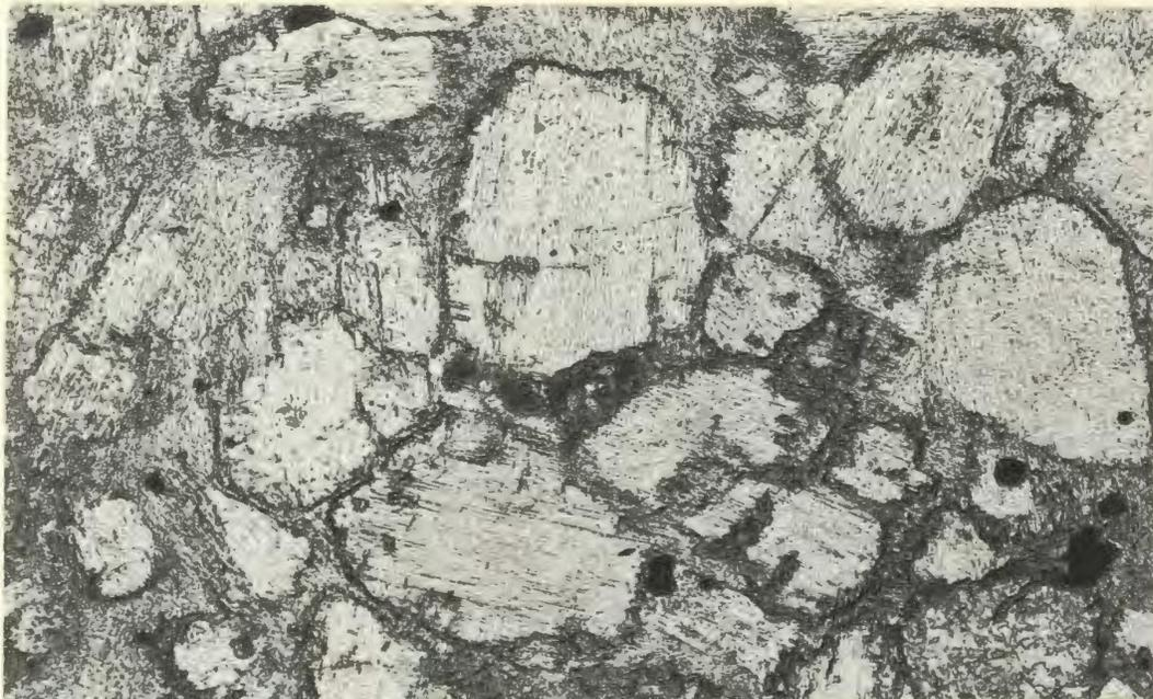
Figure 11: Photomicrograph showing bastite pseudomorphs after orthopyroxene. The pseudomorphs are altered to talc along the margins. Note the remnant cleavage in bastite. Plane polarized light (X40).
