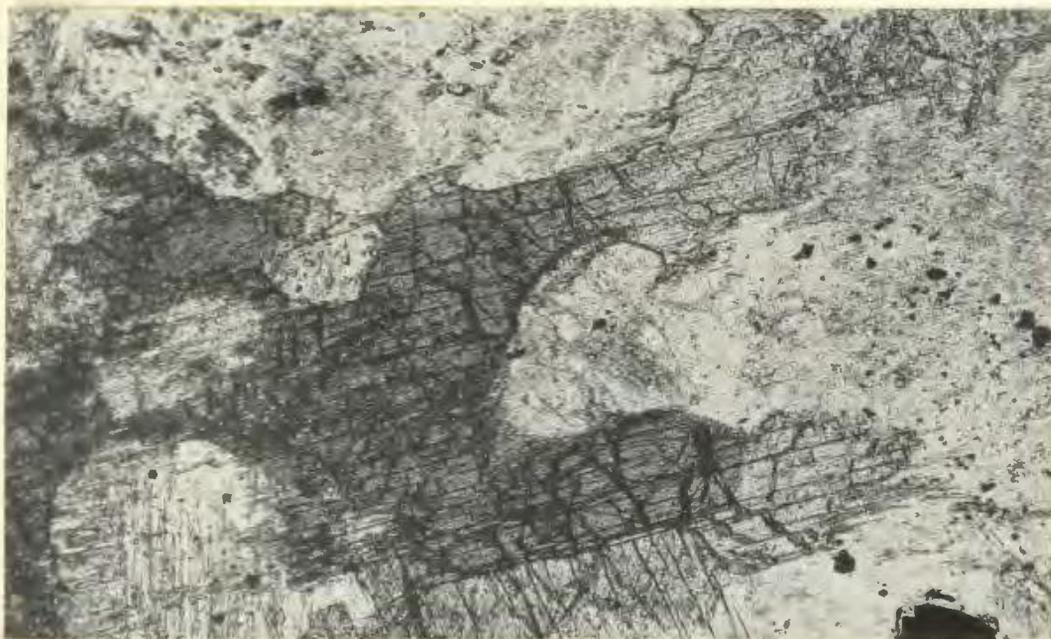
Figure 14: Photomicrograph of a thersolite sample showing intercumulate brown amphibole (secondary after clinopyroxene) grading into colourless amphibole. Plane polarized light (X40).
