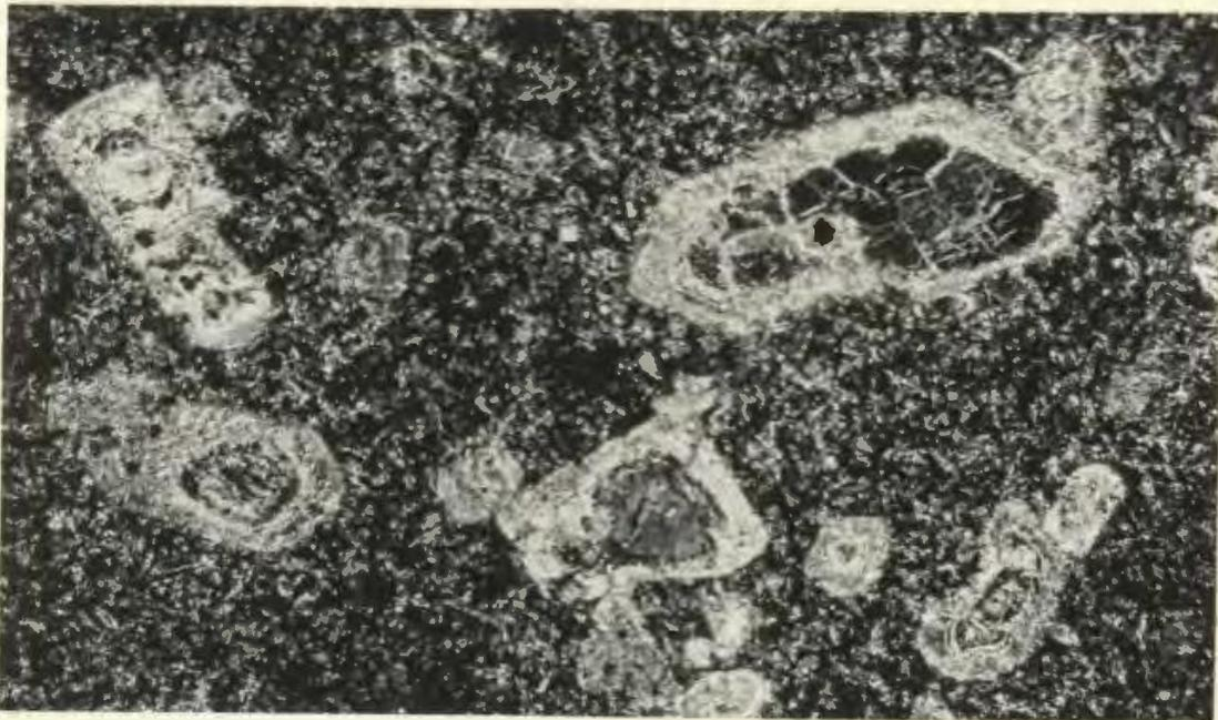
Figure 27: Photomicrograph of a porphyritic ultramafic (perknite) dyke in which pyroxene phenocrysts are altered to serpentine in the cores and to amphibole on the margins. The groundmass consists of partly uralitized pyroxene crystals. The dyke cuts layered ultramafic rocks to the south of Kitty Pond. Crossed nicols (X40).
