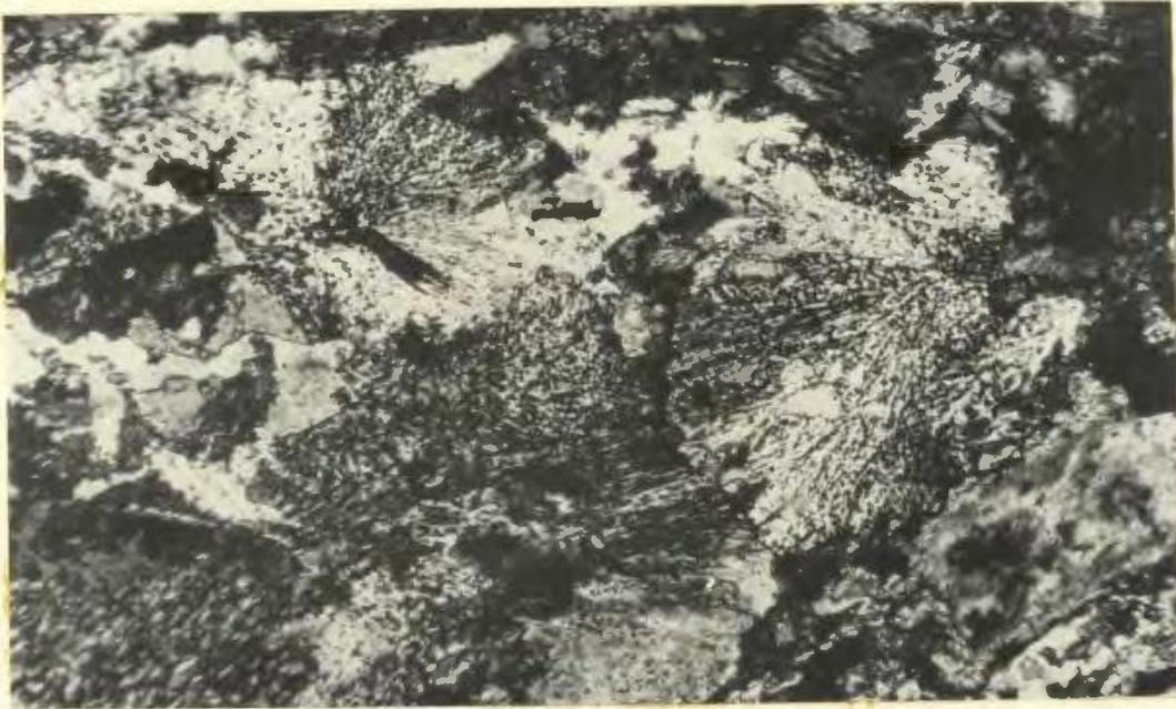
Figure 19: Photomicrograph of a gabbro sample showing the granophyric intergrowth between quartz and altered feldspar. Crossed nicols (X80).
