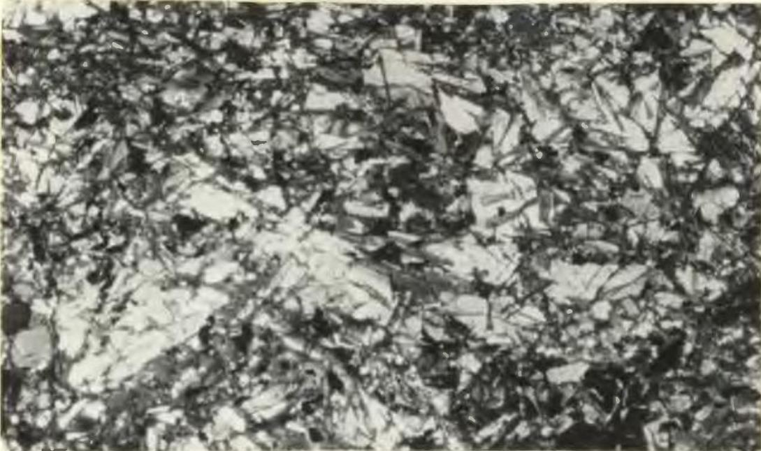
Figure 38: Photomicrograph of a typical subophitic texture in the pillow lavas of Round Harbour Basalt. Light grains are clinopyroxene, grey laths are plagioclase. Crossed nicols (X40).
