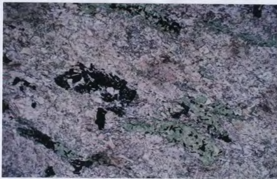
Figure 7-4 Photomicrograph from the ankerite-sericite alteration zone. Patches of chlorite (green) contain abundant rutile and ilmenite inclusions (x25).
