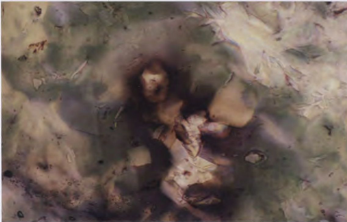
Figure 7-14 Photomicrograph of hydrothermal monazite inclusions in the chlorite-magnetite altered gabbro (x250).
