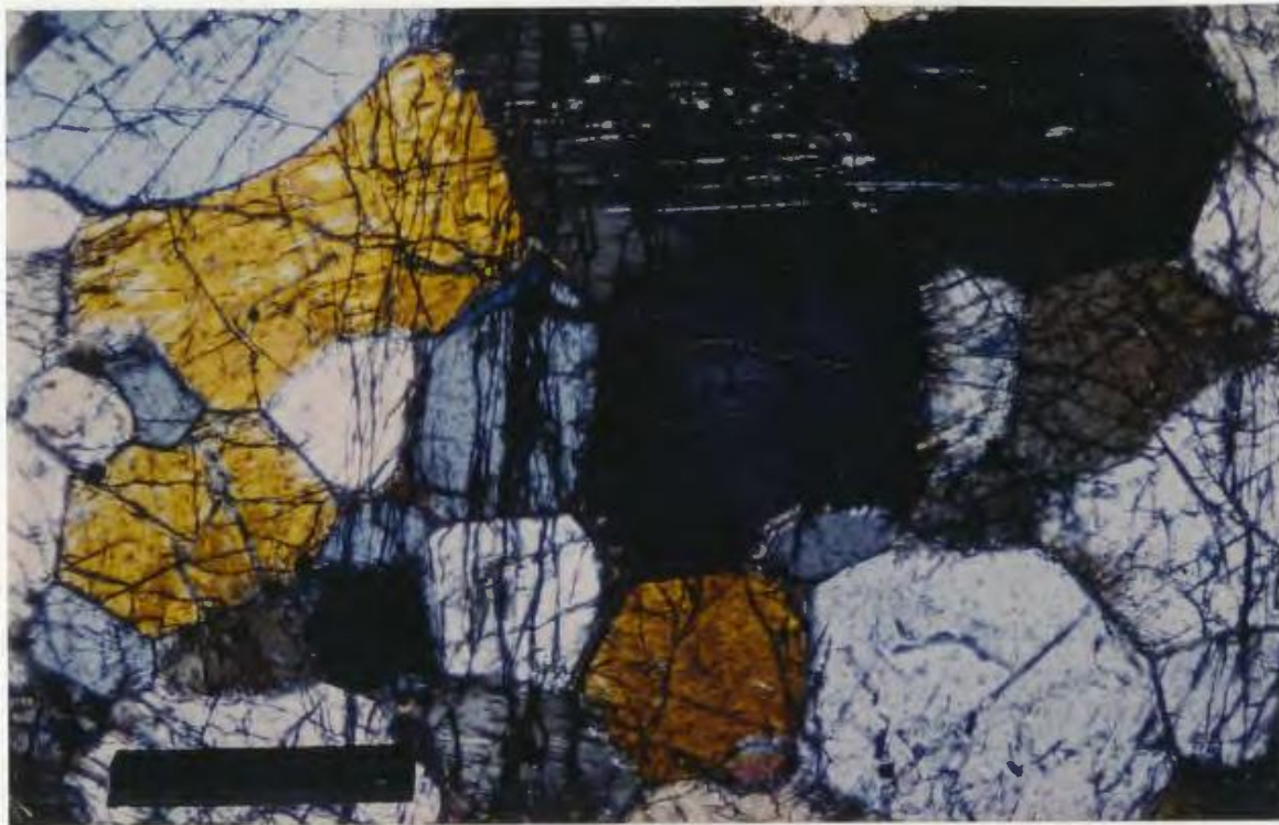
Figure 3-15: Orthopyroxene porphyroblast exhibiting development of undulose extinction and distinct equant subgrains (top right corner) in which adjacent subgrain walls (crystal lattice) are offset a few degrees ( \sim 2^\circ ). Bar scale = 1 mm.
