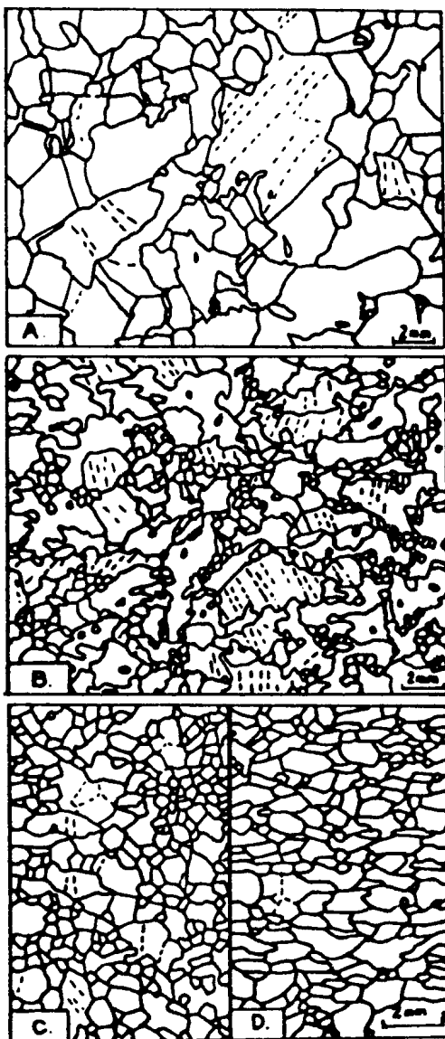
Figure 3-10: Typical microstructures of ductilely deformed peridotites: A= Protogranular: no foliation, few kinkbands, undulose extinction; B= Porphyroclastic: kinkbanded and elongate porphyroclasts recrystallized in surrounding neoblasts; C-D= Granoblastic: complete recrystallization into either equant (C) or tabular (D) neoblasts (after Gueguen and Nicolas, 1980).
