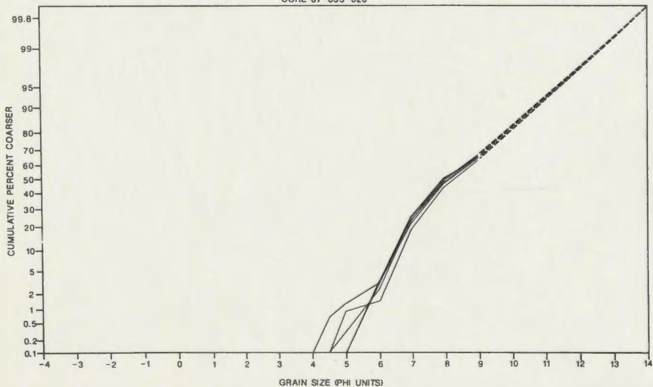
Figure 4.9. Cumulative grain size curves, plotted on probability scale ordinate, for facies 2 and 3. Data are extrapolated from 9 $\phi$  to an assumed minimum grain size of 14 $\phi$ .
