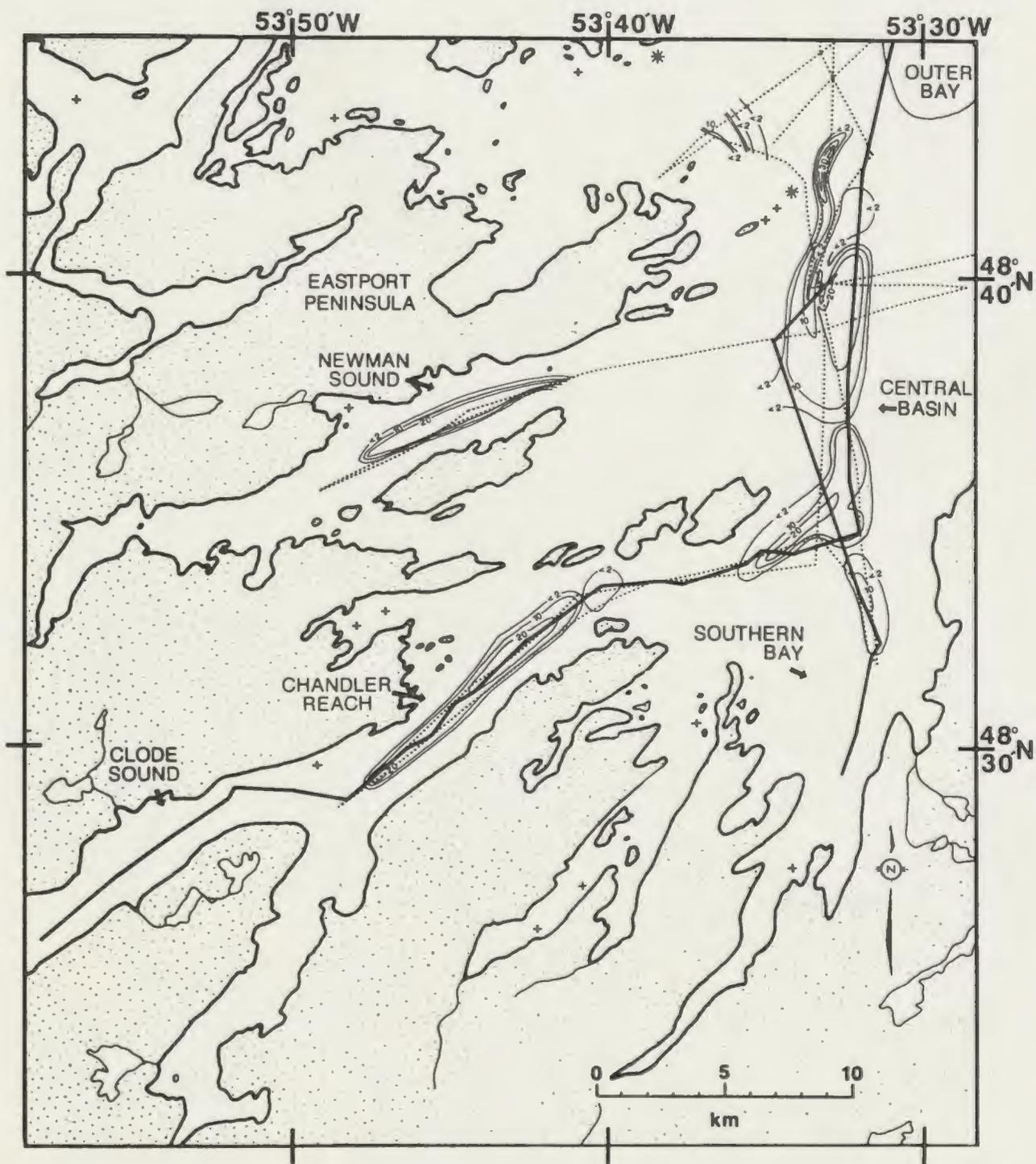
Figure 5.6. Post-glacial sediment thickness within the inner bay (seismic unit D). Contours in milliseconds two-way-travel-time.
