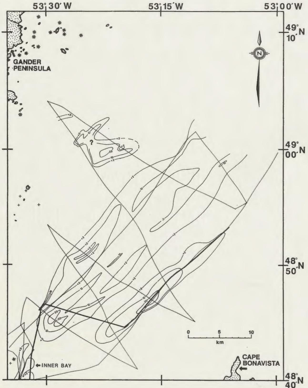
Figure 5.5. Post-glacial sediment thickness within the outer bay (seismic unit 3). Contours in milliseconds two-way-travel-time.
