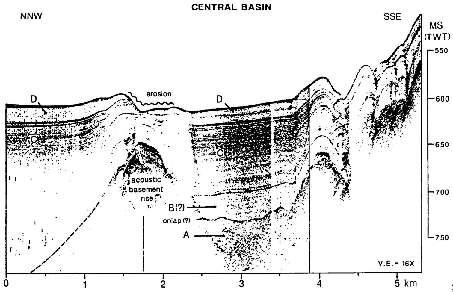
Figure 3.19. 3.5 kHz E-W profile within Central Basin. Location shown in figure 3.4. Seismic units A to D are discussed in text. Boundaries of units A and B are tentative within the main basin. Dashed line denotes continuation of acoustic basement on the basis of airgun data. V.E. = vertical exaggeration. Depth in milliseconds two-way-travel-time.
