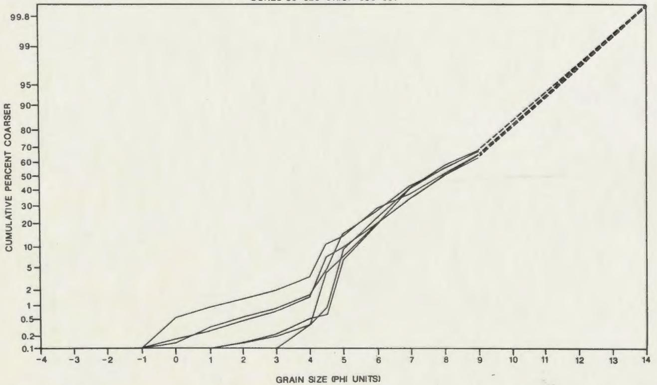
Figure 4.8. Cumulative grain size curves, plotted on probability scale ordinate, for facies 1 in inner and outer Bonavista Bay. Data are extrapolated from 9 $\phi$  to an assumed minimum grain size of 14 $\phi$ .
