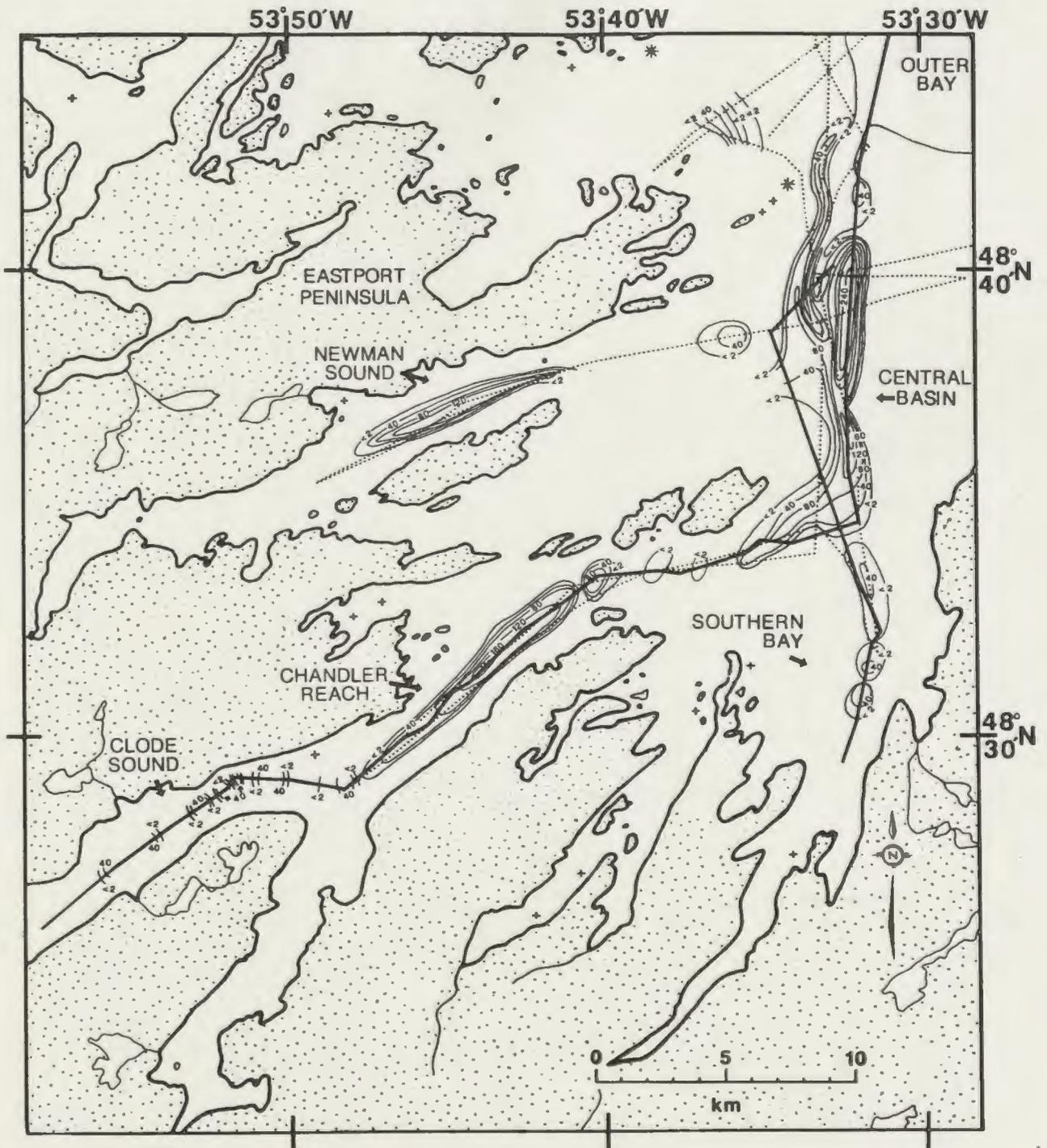
Figure 5.2. Total sediment thickness above acoustic basement within the inner bay. Contours in milliseconds two-way-travel-time. The nature of contours within Clode Sound are uncertain.
