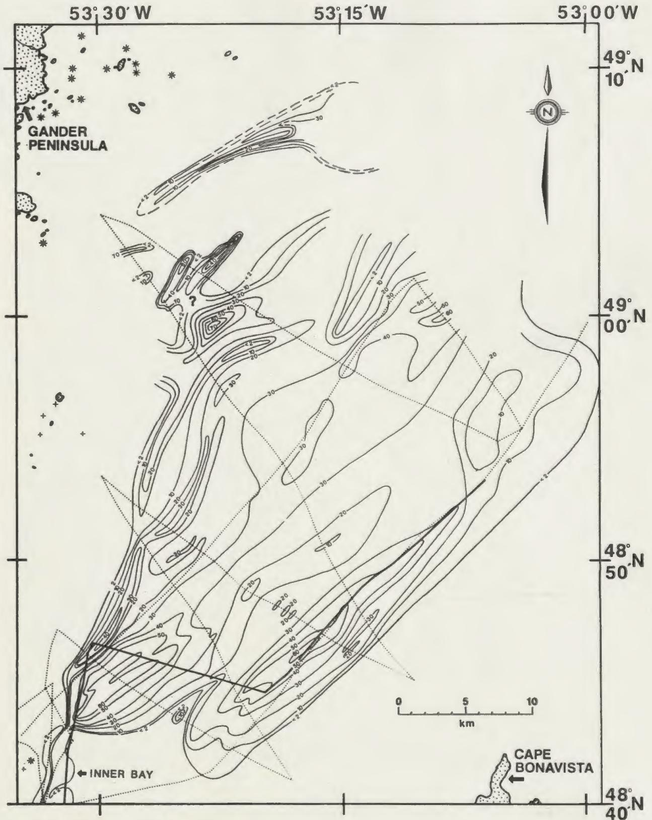
Figure 5.1. Total sediment thickness above acoustic basement within the outer bay. Contours in milliseconds two-way-travel-time. Dashed contour to the north denotes area of uncertain correlation.
