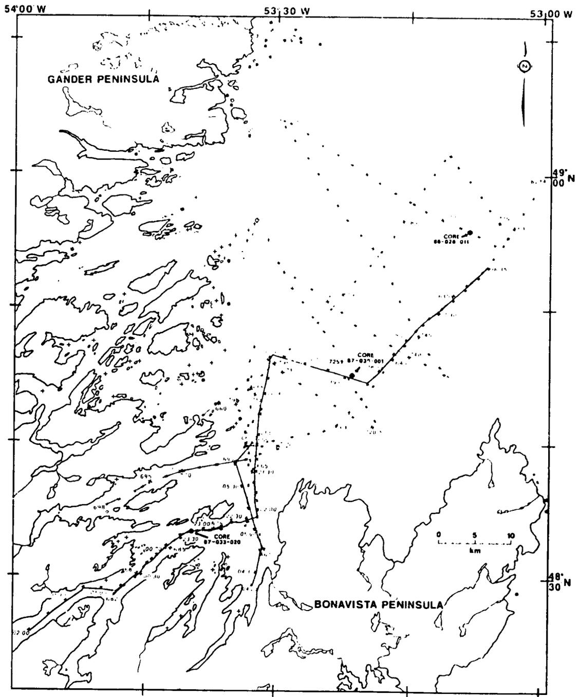
Figure 2.1. Map of the primary seismic survey coverage and core sites within the study area.
