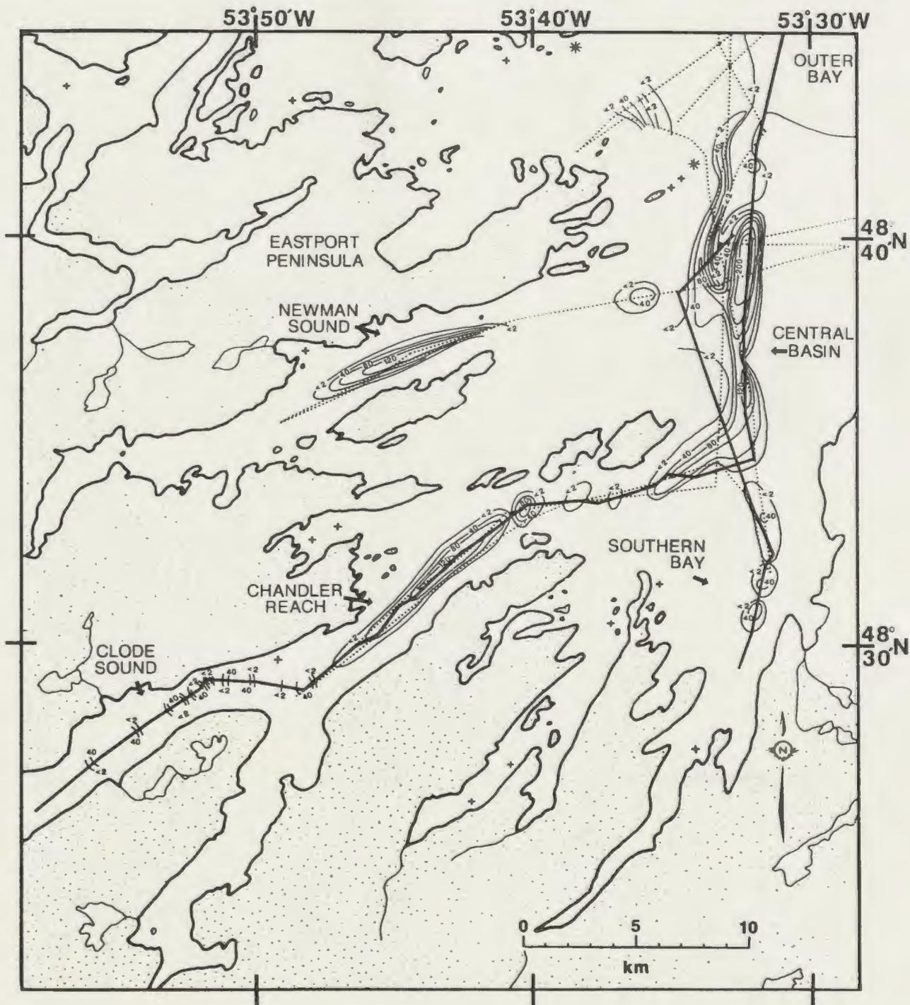
Figure 5.4. Glacial and proglacial sediment thickness within the inner bay (seismic units A to C). Contours in milliseconds two-way-travel-time. The nature of contours within Clode Sound are uncertain.
