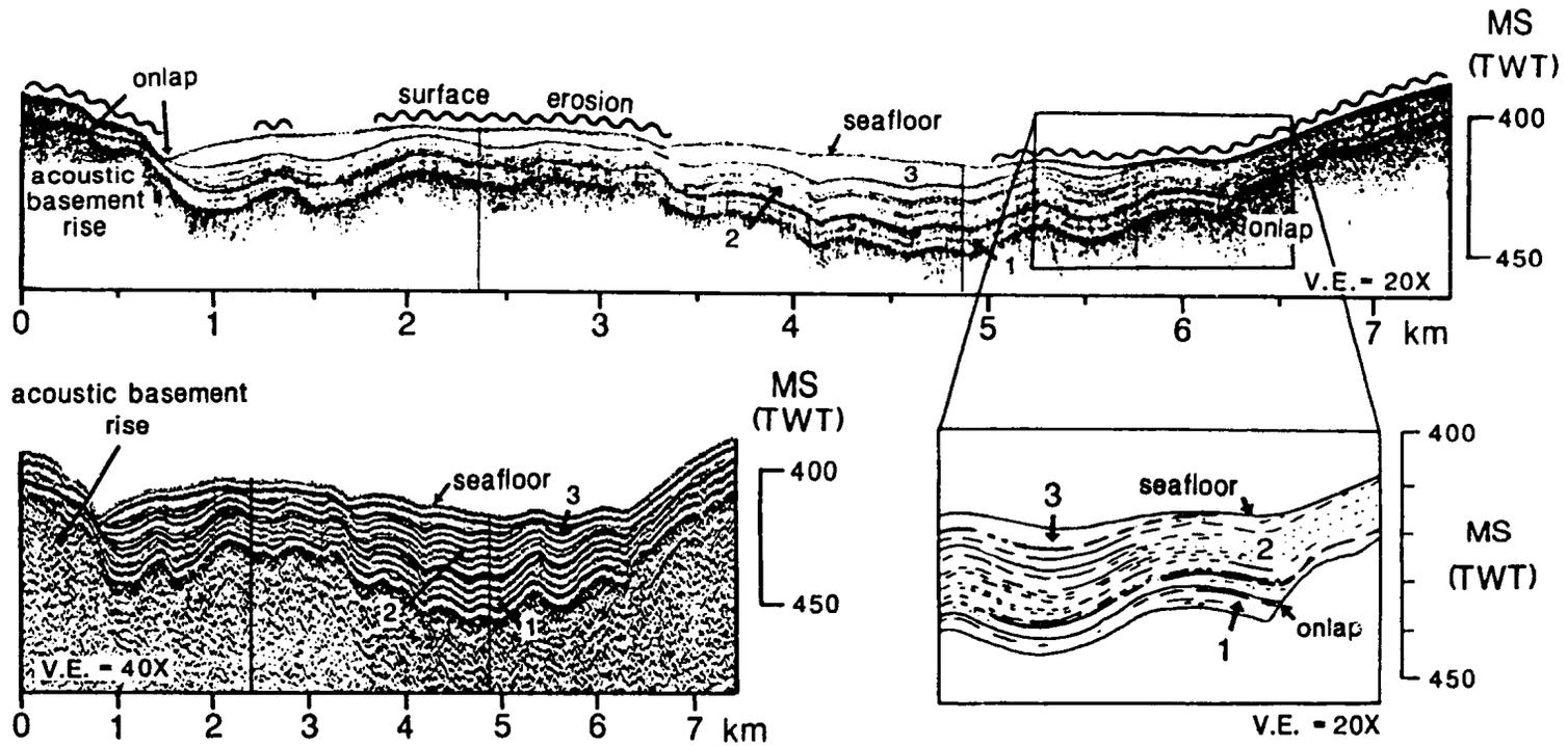
Figure 3.9. 3.5 kHz and airgun profiles within the Western Basin. Location shown in figure 3.4. Seismic units 1 to 3 are discussed in text. Dashed line denotes tentative seismic unit boundaries. V.E. = vertical exaggeration. Depth in milliseconds two-way-travel-time.
