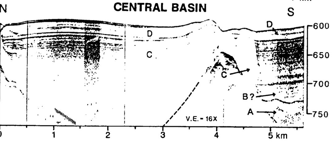
Figure 3.12. Tentative correlation of seismic units observed in airgun data from the main basins of inner Bonavista Bay. Basin locations illustrated in figure 3.1. Chandler Reach and Newman Sound data from C.S.S Dawson cruise 86-026; Central Basin data from C.S.S. Hudson cruise 87-033. V.E. = vertical exaggeration. Depth in milliseconds two-way-travel-time.
