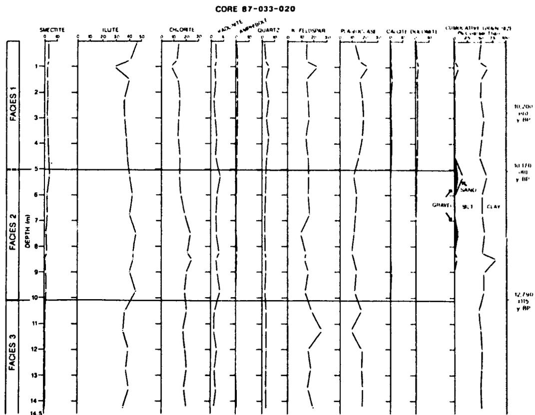
Figure 4.6. Relative abundances of clay and non-clay minerals within the clay-sized fraction, as well as cumulative grain size data, plotted against depth in core 87-033-020. Data for each sample normalized to 100%.
