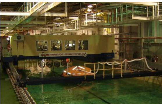
Figure 1 Liferaft setup between the towing carriage and the service carriage at NRC-IOT
