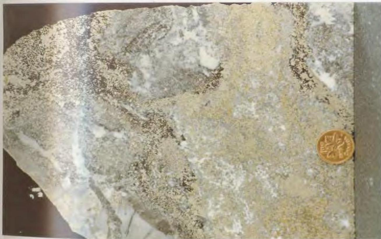
Plate 4-1: Stockwork mineralization, Lucky Strike area.
