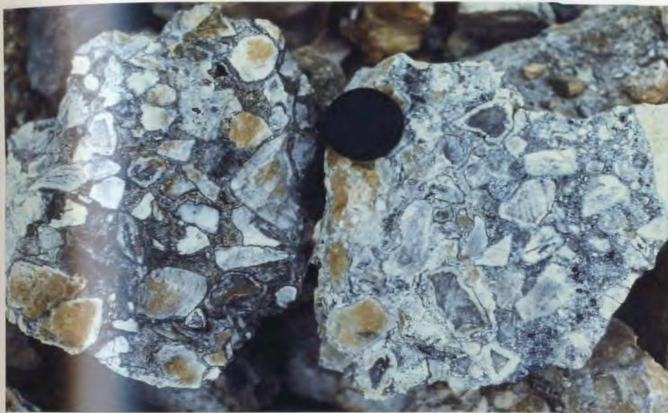
Plate 4-16: Motoyama volcanic breccia, Kosaka Mine. Note altered rims on rhyolite fragments, similar to those occurring at Buchans.
