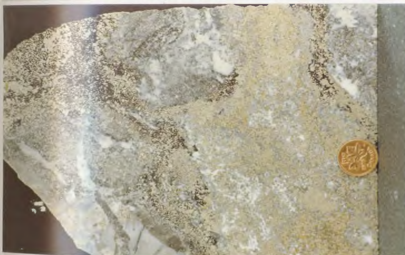
Plate 4-1: Stockwork mineralization, Lucky Strike area. Top; chalcopyrite-pyrite veinlets cutting sulphide-impregnated chloritized host. Bottom; silicified and chloritized stockwork.
