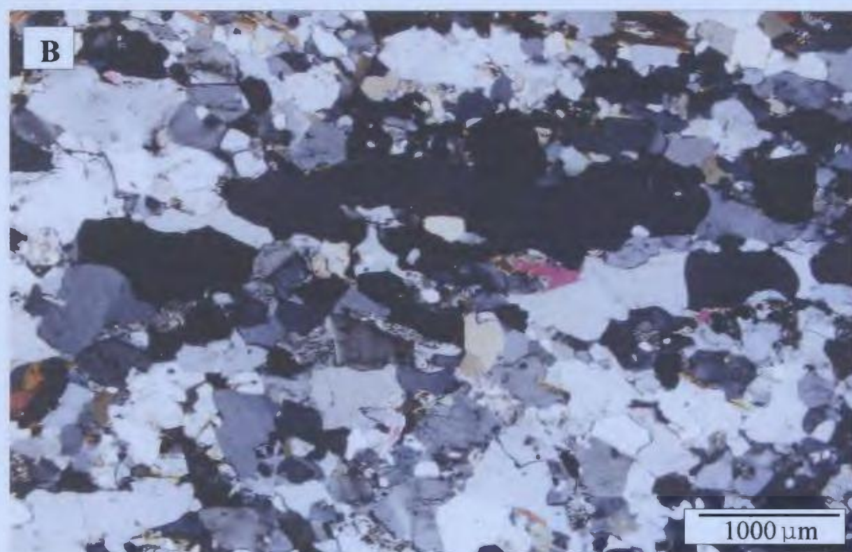
Plate 4.1: Coarse-grained areas dominated by quartz ribbons, probably representing restite (Sample 100). (A) plane polarized light and (B) cross polarized light.
