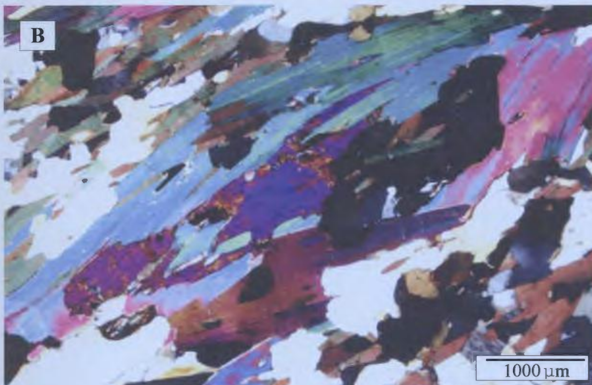
Plate 5.8: Retrograde muscovite aggregates corroding kyanite and quartz (sample 31A). These aggregates also contain relict garnet inclusions. Lines A-B and C-D indicate paths of microprobe analyses across a relict garnet (See Figure 5.7). (A) plane polarized light and (B) cross polarized light.
