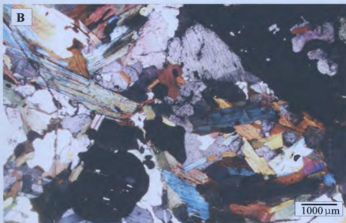
Plate 8.9: Primary muscovite (sample 70). (A) plane polarized light and (B) cross polarized light.
