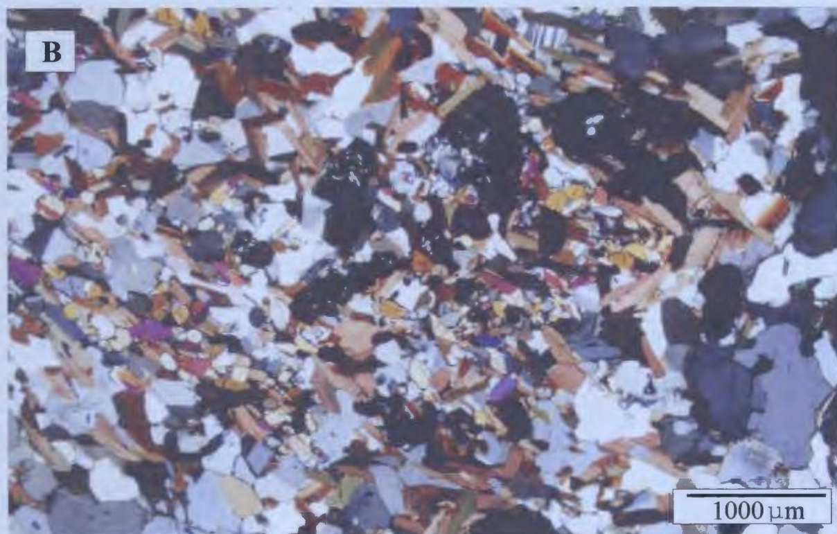
Plate 4.6: Garnet relic corroded by kyanite + biotite + plagioclase + quartz aggregates which probably formed during melt crystallization (sample 100). (A) plane polarized light and (B) cross polarized light.
