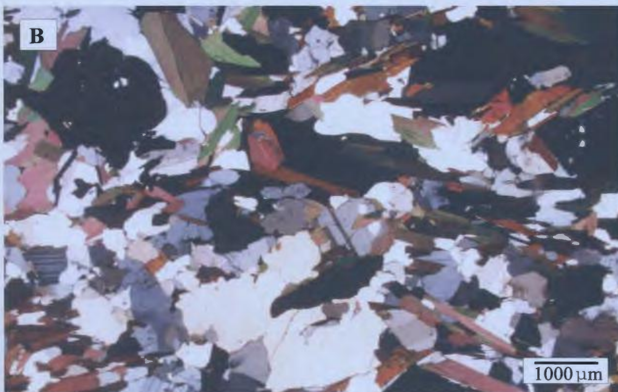
Plate 8.8: Matrix consisting of plagioclase, quartz and biotite (sample 9). (A) plane polarized light and (B) cross polarized light.
