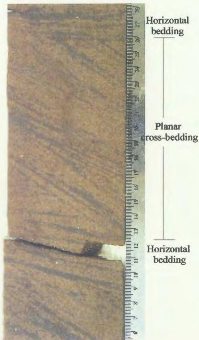
Figure 3.3. Planar cross bedded, medium grained sandstone, characteristic of facies H3. Also shown here is the truncation of horizontal bedding by planar cross beds. Photomicrographs shown on the right show the poorly to moderately well sorted, very fine to very coarse grained quartzarenites characteristic of a portion of the reservoir sands of facies H3. Photomicrographs taken by corelabs are courtesy of HMDC.
