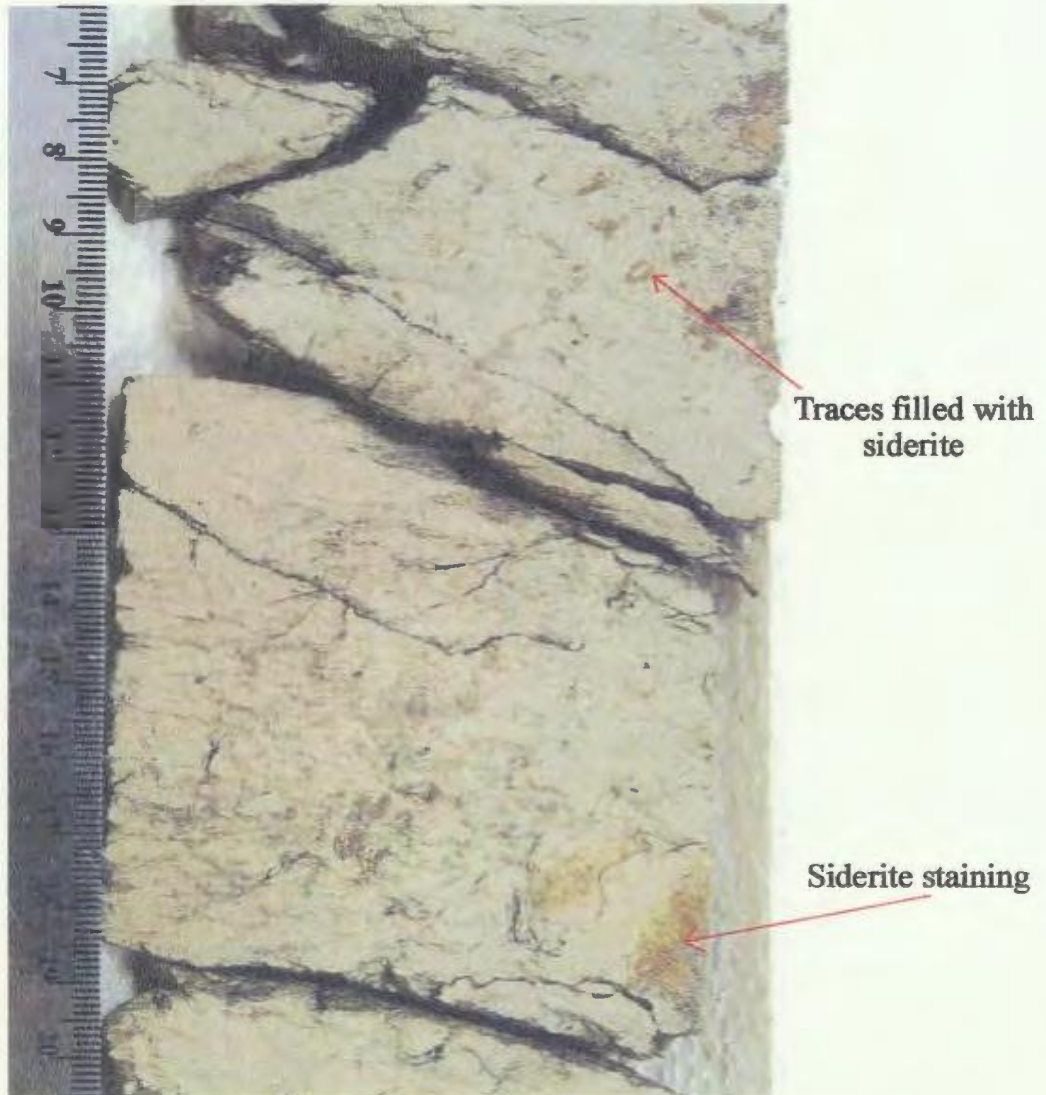
Figure 3.11. Rooted shale characteristic of facies H11. These shales exhibit common to abundant rooting and contain siderite. The shales range from grey to slightly greenish-red in color. The siderite occurs as staining and is also seen within root traces.
