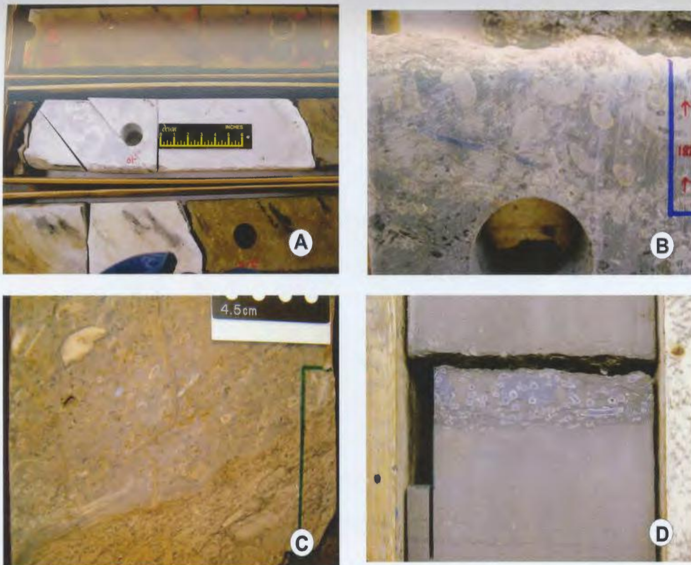
Figure 3.12: Varying cementation intensities found in the Ben Nevis Formation. A. Very well cemented concretion B-07_4, Core 2, Box61, B. Well cemented, F-04, Core 3, Box 31, C: Moderately cemented, F-04, Core 1, Box 38 and D. Partial cementation, F-04, Core 2, Box 52.
