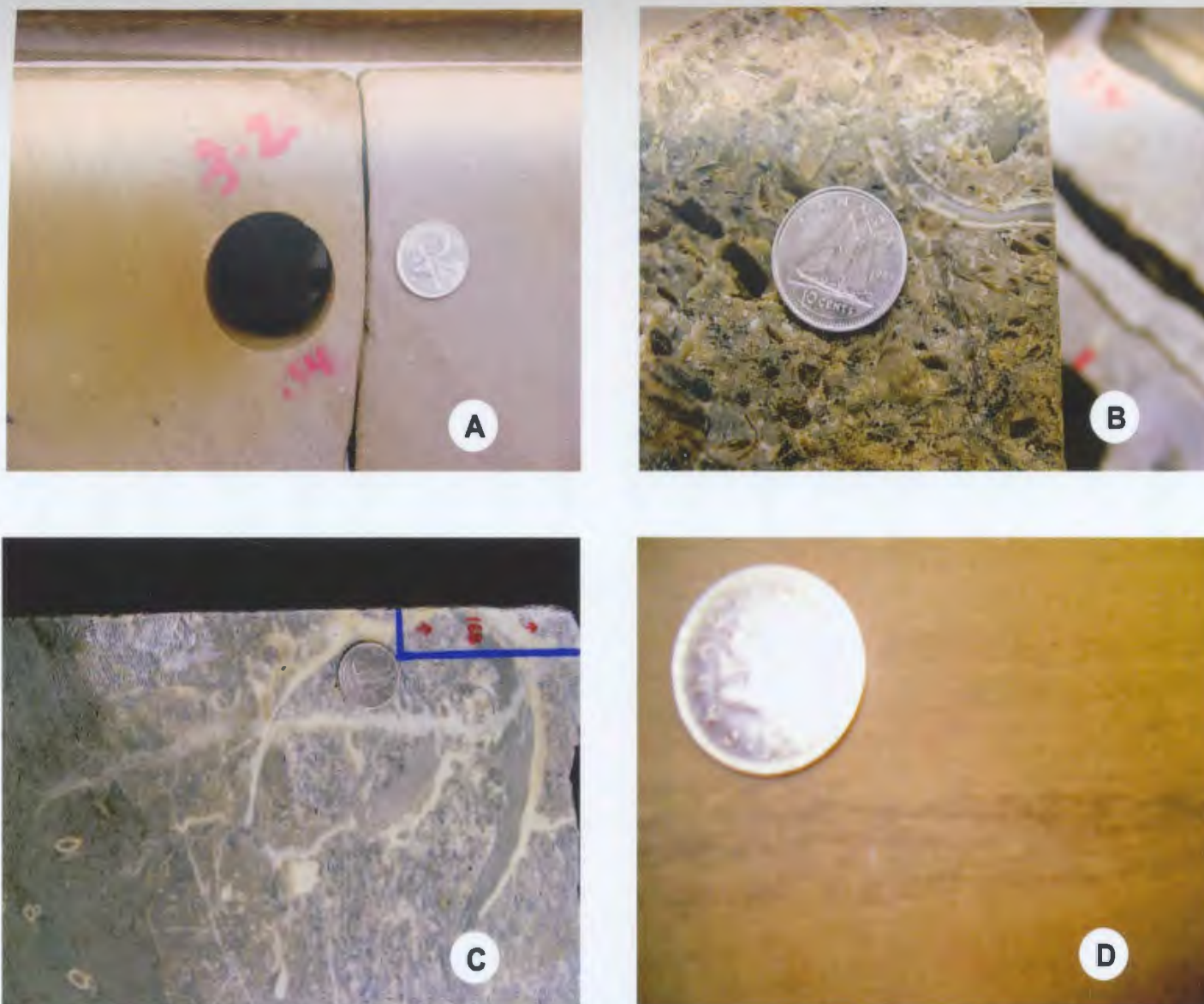
Figure 3.6: Characteristics of the main Ben Nevis sandstone A. Low Angle Cross Bedding, B-07_4, Core 1, Box 3; B. Longitudinal section of Serpulid Worm Tube B-07_4, Core 2, Box 6; C. Large Bivalve, B-07_4, Core 2, Box 22; D. Thin Black Partially Dissolved Shells, B-07_4, Core 1, Box 62.
