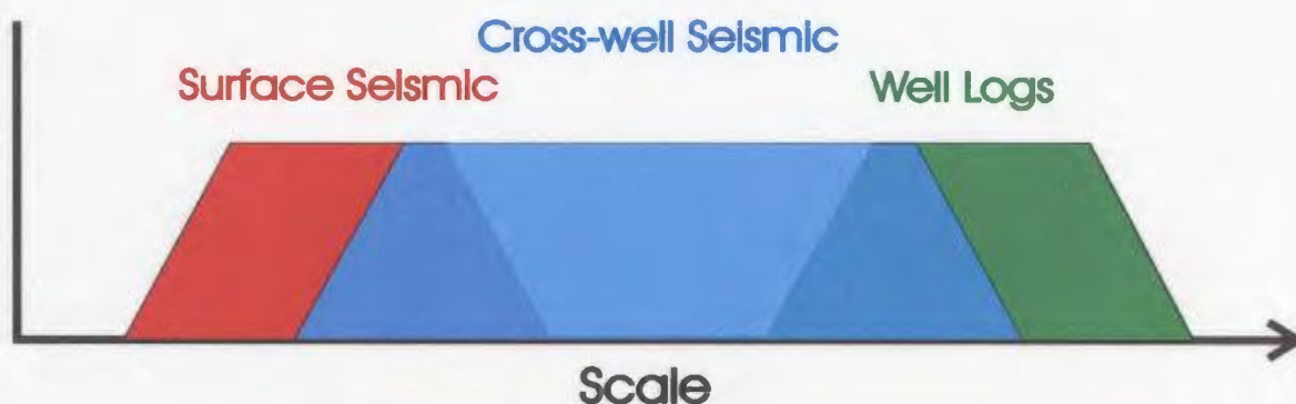
Figure 1.1: Schematic showing how cross-well data bridges the resolution gap between surface seismic data and well log data.
