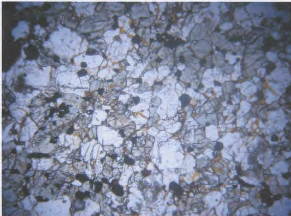
Plate 2-43. Photomicrograph of sample BS 6a, collected from a layer adjacent to contact with monzonite on the south side of Nain Bay. Plane polarized light. The texture of this rock is identical to medium-grained ferrogabbroid, but it has silica content much higher than typical ferrogabbroid. Field of view ca. 5.5 mm.
