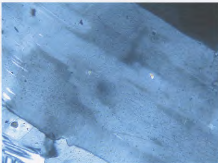
Plate 2-16. Photomicrograph of troctolite sample BS 5d, north of Nain Bay. Crossed polars. Tiny, dark needlelike inclusions in plagioclase. The abundance of the needles is associated with chemical zoning in the grain. Chemical zoning is demarcated by grain darkness. Field of view ca. 1.5 mm.
