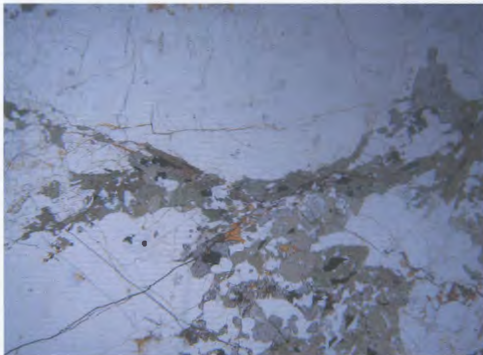
Plate 2-54. Photomicrograph of monzonite sample BII 68. Plane polarized light. Apparent deformation of ductile mafic material around a large mesoperthite crystal in monzonite. Field of view ca. 5.5 mm.
