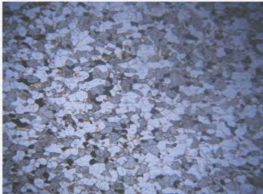
Plate 2-38. Photomicrograph of ferrogabbroid sample LBE 42, north of Nain Bay. Plane polarized light. The anhedral, equigranular texture of the fine-grained ferrogabbroids is well-illustrated. Note the distinct alignment of both plagioclase (white mineral) and pyroxene (darker mineral). The opaque mineral is magnetite. Field of view ca. 5.5 mm.
