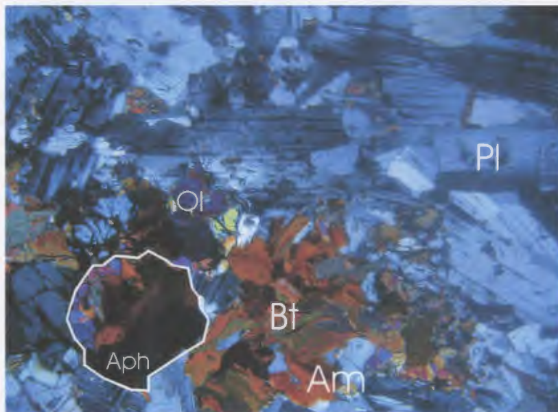
Plate 2-58a. Photomicrograph of sample BIII 19. Crossed polars. Troctolite near its contact with monzonite on the west end of Barth Island. Notice the coarse plagioclase (Pl). The white outline delineates amphibole as a pseudomorph (Aph) of olivine (Ol). A piece of the original olivine crystal is preserved at the left side of the amphibole crystal. Much of the biotite (Bt) and amphibole (Am) is secondary. Field of view ca. 5.5 mm.
