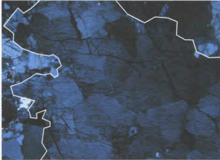
Plate 2-49. Photomicrograph of monzonite sample BS 6b. Crossed polars. Photo of undulatory extinction in a large mesoperthite grain, which signifies the development of subgrains. White outline marks the grain boundary, subgrains are delineated by the different brightnesses in the grain. Field of view ca. 5.5 mm.
