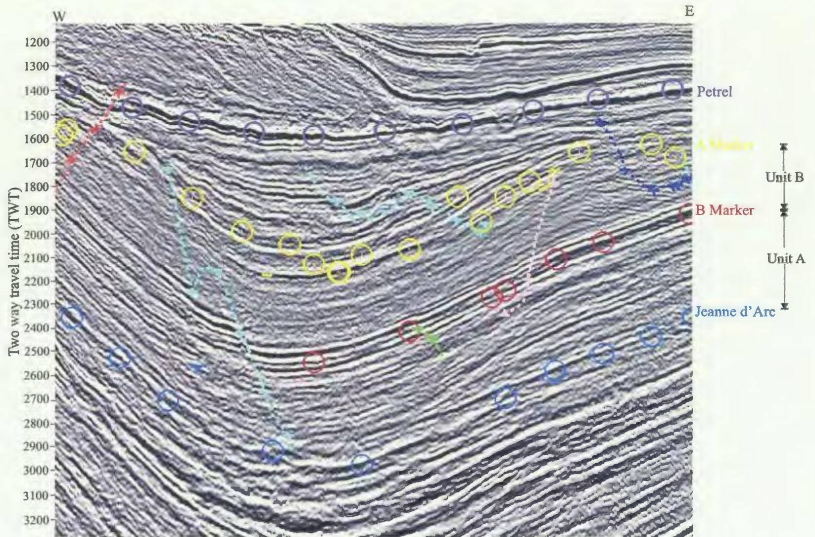
Figure 3.4. W-E oriented seismic line shows the broadly synclinal architecture of the Petrel Member, and succession below, which demonstrate the curved architecture of the Cape Pine syncline. The Petrel event, has a synclinal shape (200 ms TWT vertical difference), which curves toward eastern and western structural highs. See Figure 3.2 for line location. The colored circles indicate cross line correlation points of seismic stratigraphic surfaces.
