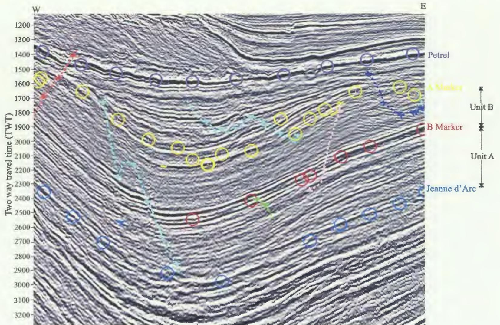
**Figure 3.4.** W-E oriented seismic line shows the broadly synclinal architecture of the Petrel Member, and succession below, which demonstrate the curved architecture of the Cape Pine syncline. The Petrel event, has a synclinal shape (200 ms TWT vertical difference), which curves toward eastern and western structural highs. See Figure 3.2 for line location. The colored circles indicate cross line correlation points of seismic stratigraphic surfaces.
