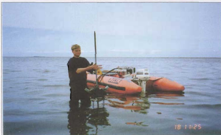
Split spoon retrieval with hydraulic jack, core location 6 (washover).
