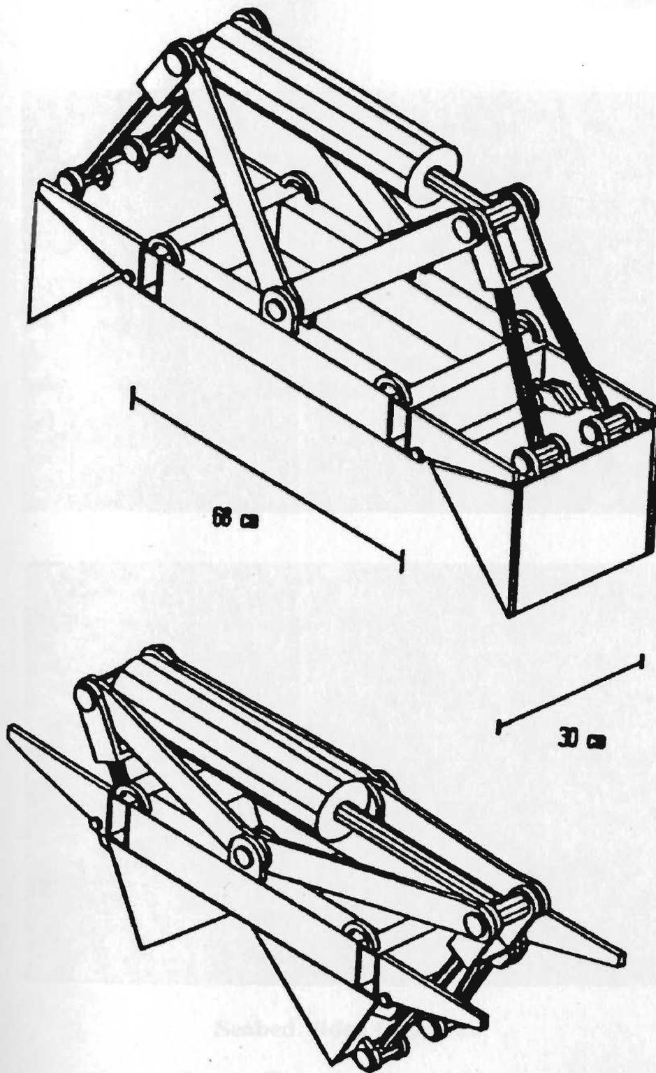
**Figure 2.58 :** Scott / C-CORE Hydraulically-Actuated Dual Bucket Sampler
