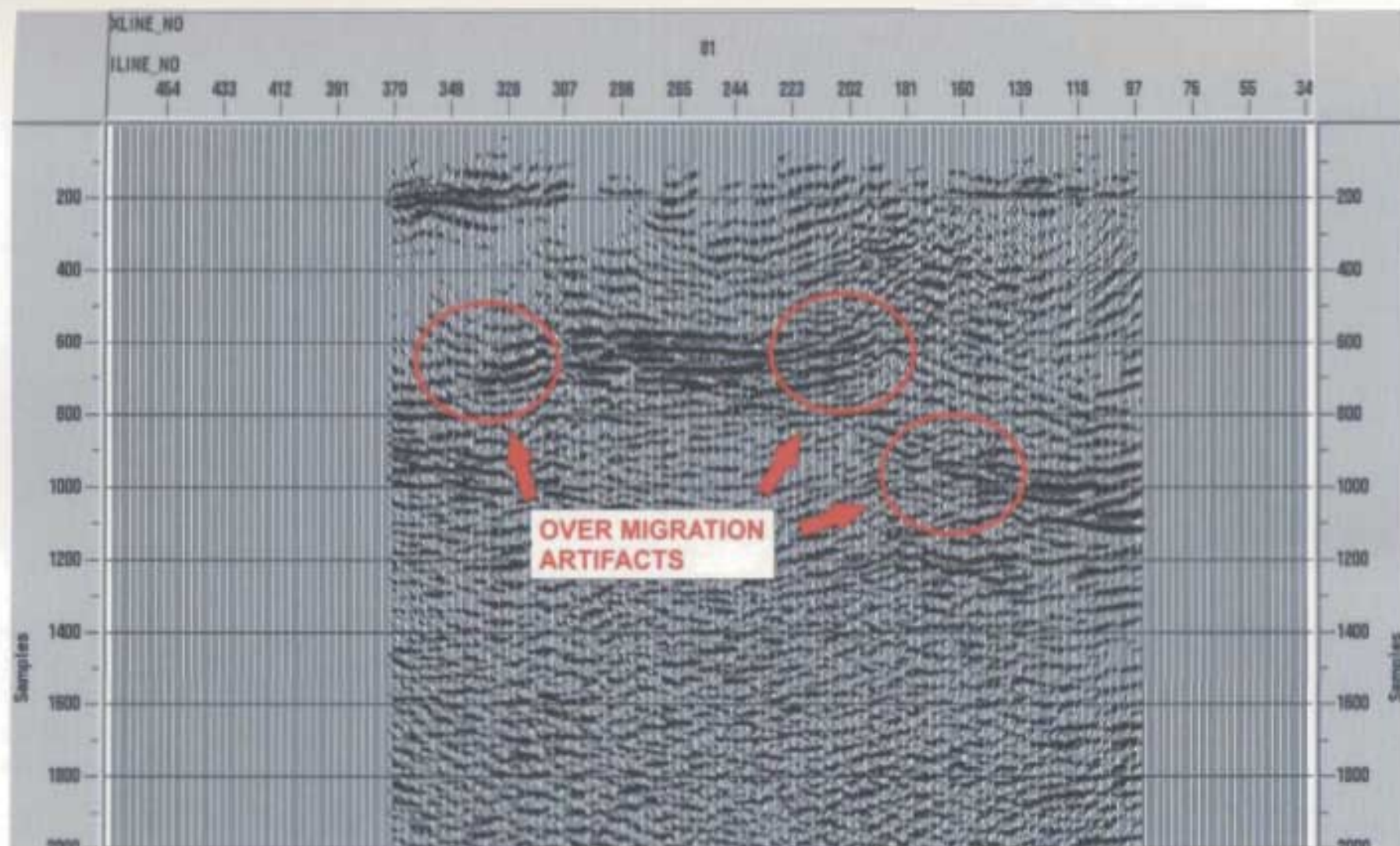
Figure 5.27b. Xline 81 Stolt migrated using a constant velocity of 2000m/s interval velocity function. Note the presence of overmigration artifacts that were not visible on 5.26a.
