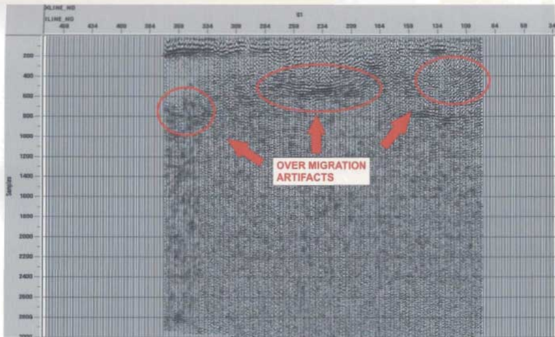
Figure 5.28b. Xline 81 Stolt migrated using a constant velocity of 2000m/s interval velocity function. Note the presence of excessive overmigration artifacts.
