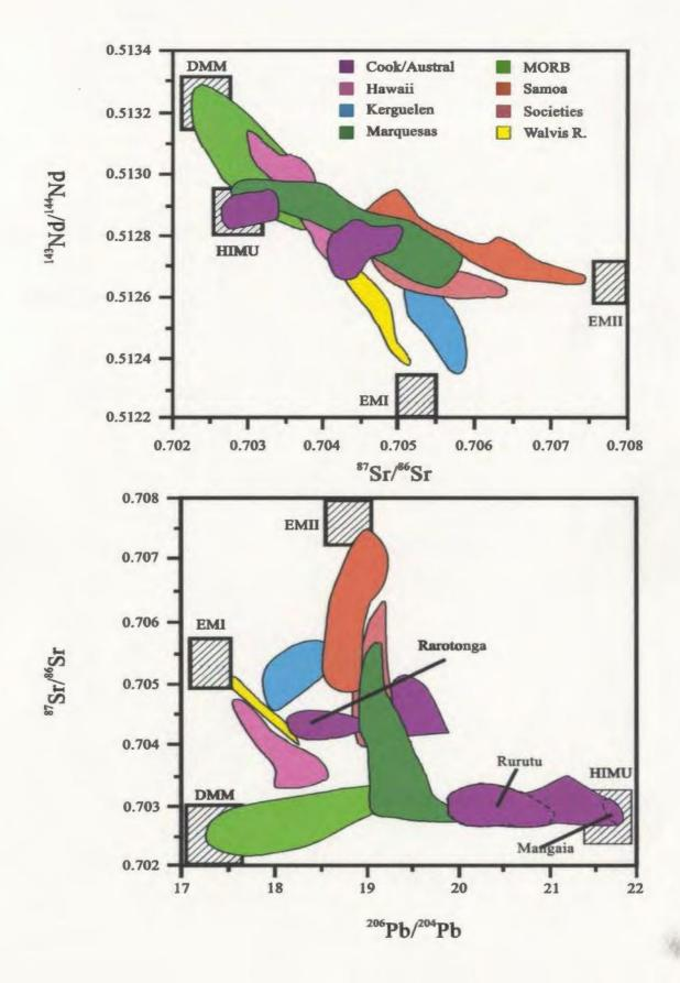
**Figure 2.3:** Isotopic variations for oceanic basalts in the South Pacific. Hypothetical mantle end-members are shown for reference (after Staudigel et al., 1984).
