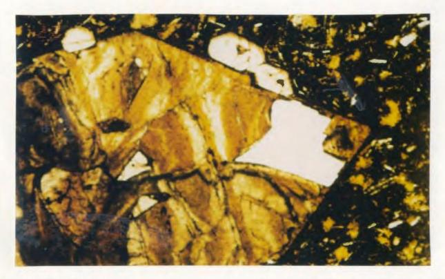
Figure 3.12: Olivine showing extensive serpentinization (R83). Crossed nicols. Field of view is 2mm
