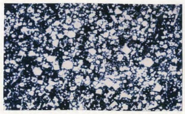
Figure 3.28: Relitively phenocryst rich foidal phonolite (R38). Crossed nicols. Field of view 2mm.
