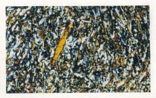
Figure 3.20: Abundant kaersutite phenocrysts in sample R56. Crossed nicols. Field of view is 1mm.
