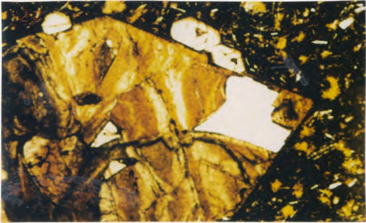
Figure 3.12: Olivine showing extensive serpentinization (R83). Crossed nicols. Field of view is 2mm
