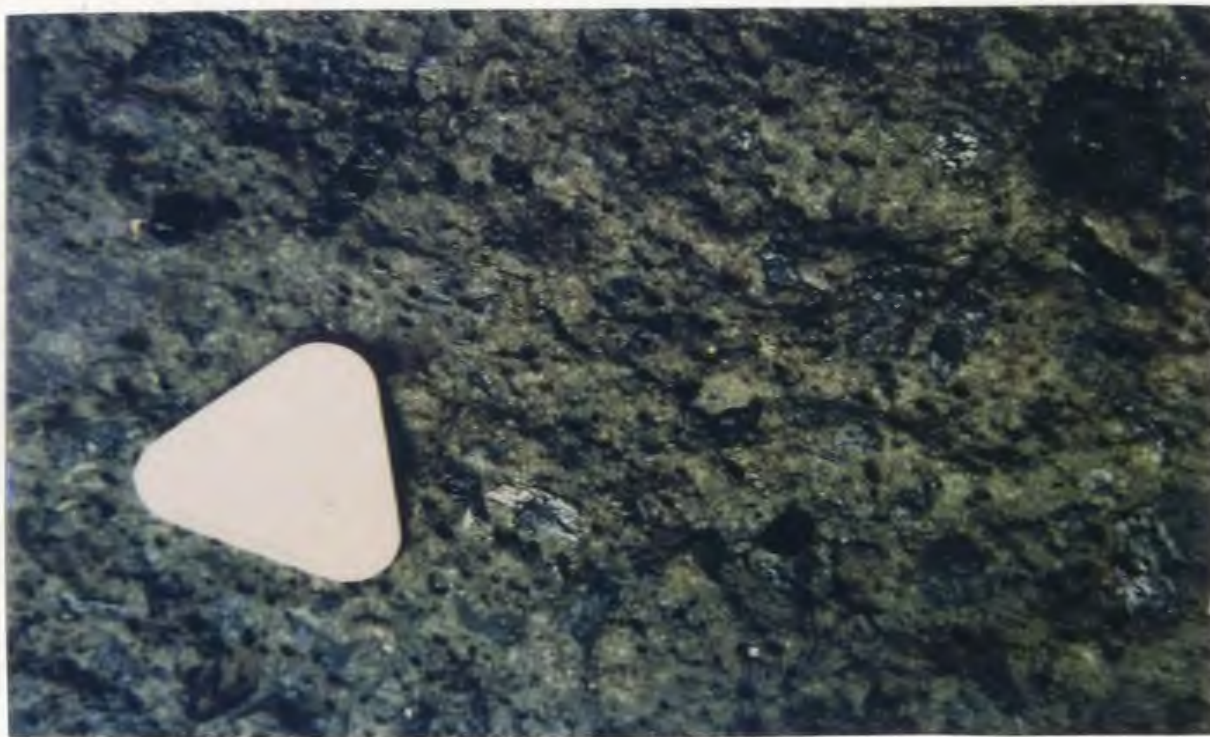
Figure 3.8: Type I ankaramite sample. Coin has approximately 1cm sides.
