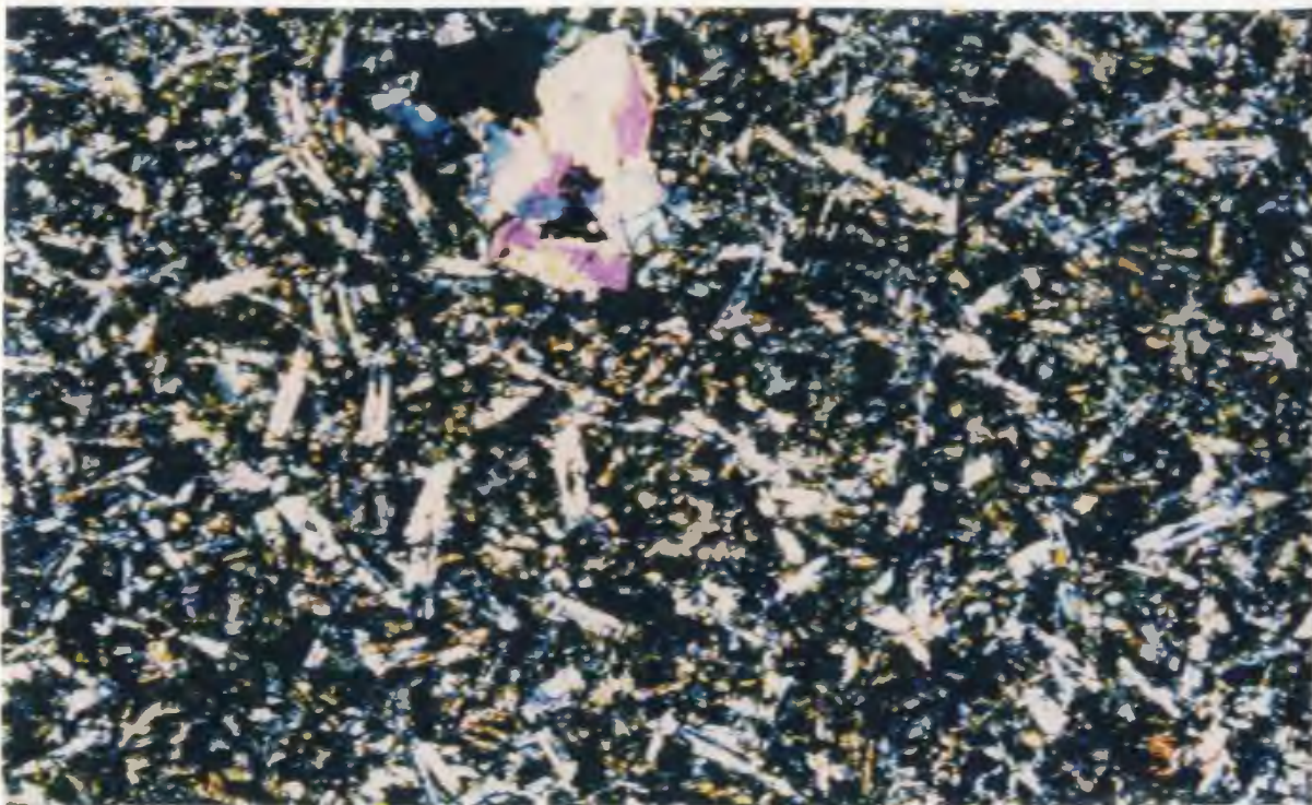
Figure 3.19: Photomicrograph of basalt (R78). Crossed nicols. Field of view is 2mm.
