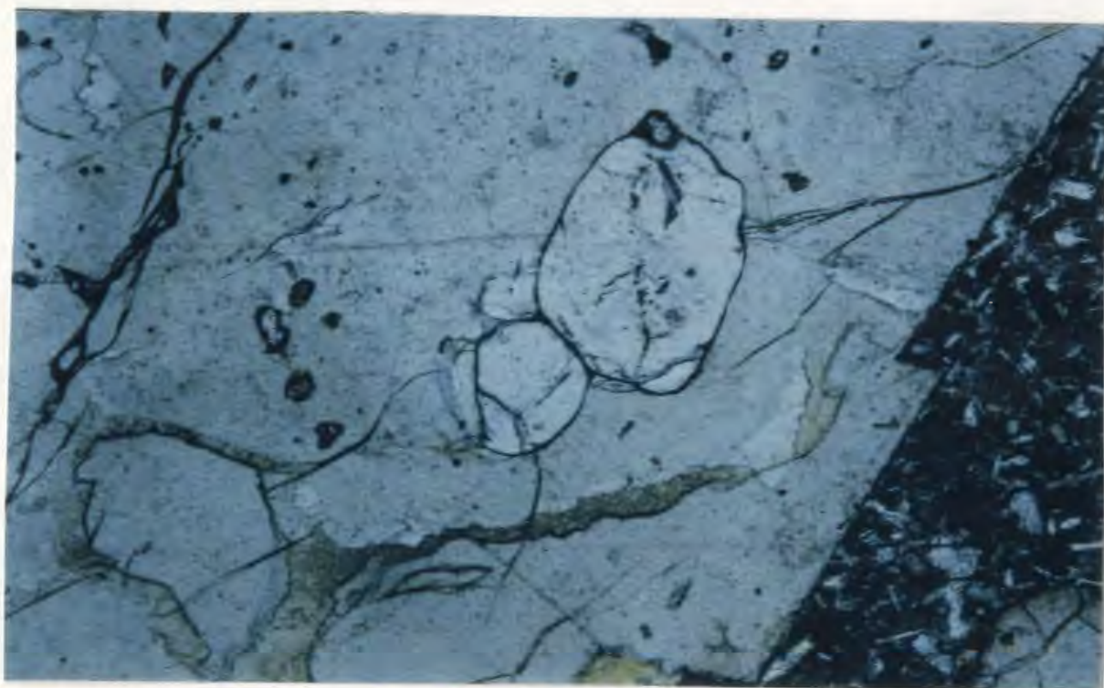
Figure 3.17: Photomicrograph of anhedral olivines in pyroxene phenocryst (R40) Plane polarized light. Field of view is 1mm.
