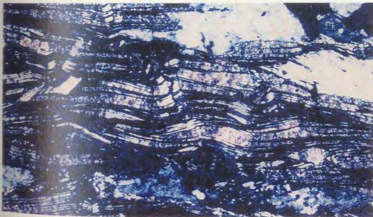
Plate 8: Photomicrograph of F4 kink folds affecting muscovite in the matrix of the Mischief Mélange. View is 10 mm across. Site 8 on Map 1.
