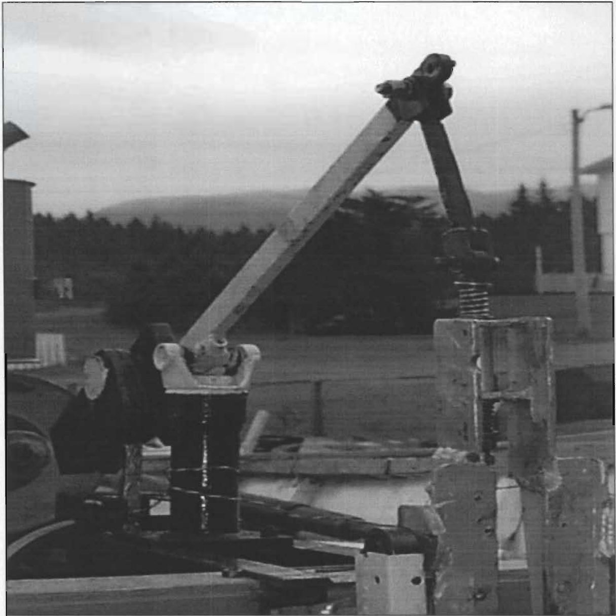
Figure 3. 24 Lever arm fully extended and connected to the eyebolt of the slider assembly
