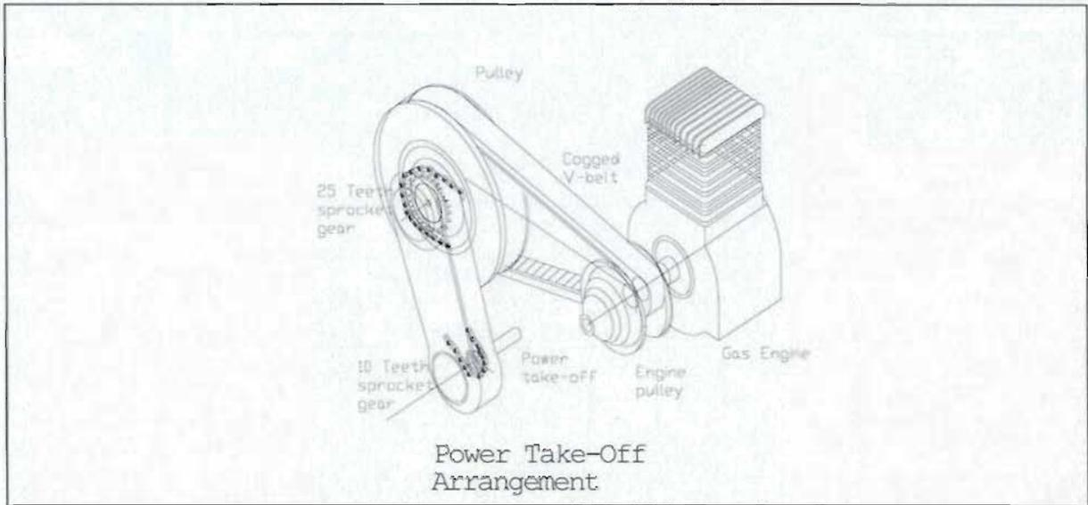
**Figure 3. 11 Installation assembly for pulley and sprocket gears**
