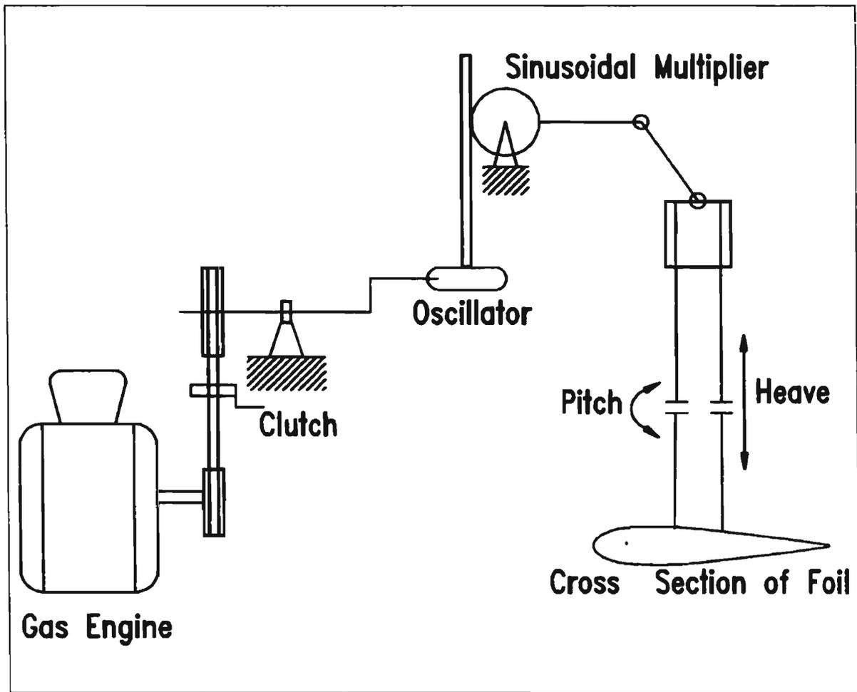
**Figure 3.1 Schematic drawing of the foil propulsion system**
