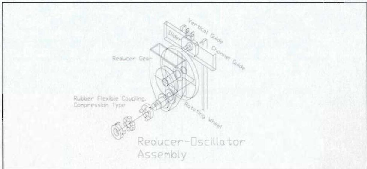
**Figure 3. 10 Installation assembly of coupling, reducer gear, and oscillator mechanism**
