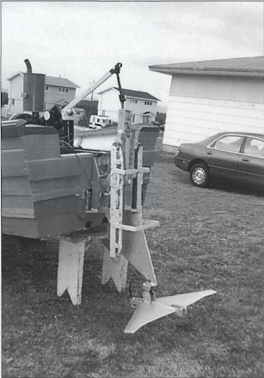
**Figure 4. 2 Design foil #2 in pre-test position**
