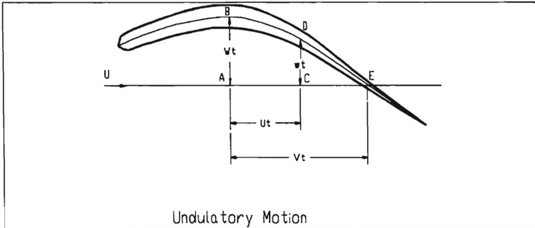
**Figure 1. 1 Undulating body**
