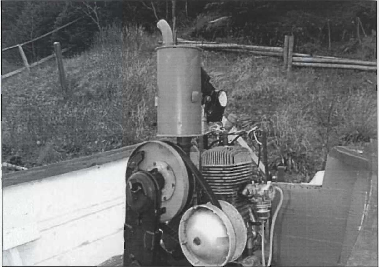
**Figure 3. 22 Drive assembly in place with fitted muffler**
