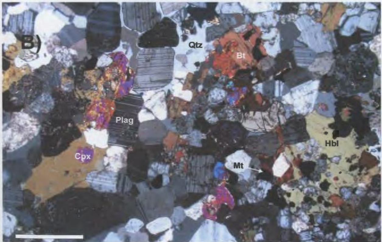
Plate 2.16. U-Pb sample DDH-496-549 (meta-tonalite) from Voisey's Bay, Labrador. A) Drill core sample. B) Photomicrograph in cross polarized light.
