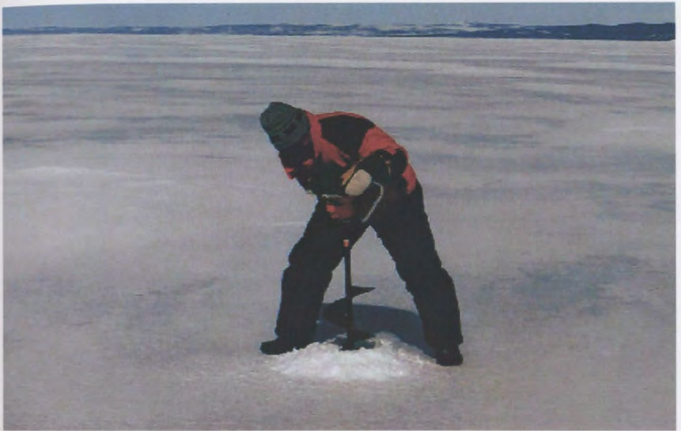
Photo 2. Drilling through the ice with a 10" gas powered ice auger on Red Indian Lake.
