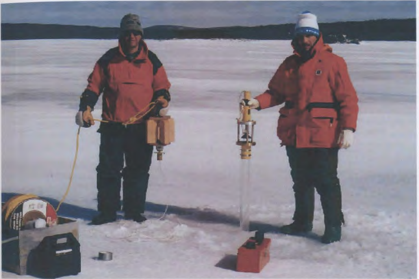
Photo 1. K.B. Gravity Corer equipped with a Deep Water Operating Kit. The Lexan tube is attached to the core head which contains the plunger mechanism. The core head is attached to the Deep Water Operating Kit via the metal weight. The Deep Water Operating Kit is attached to the large coil of \frac{1}{2} inch nylon rope. Photograph is of Al Thompson (left) and myself on Red Indian Lake.
