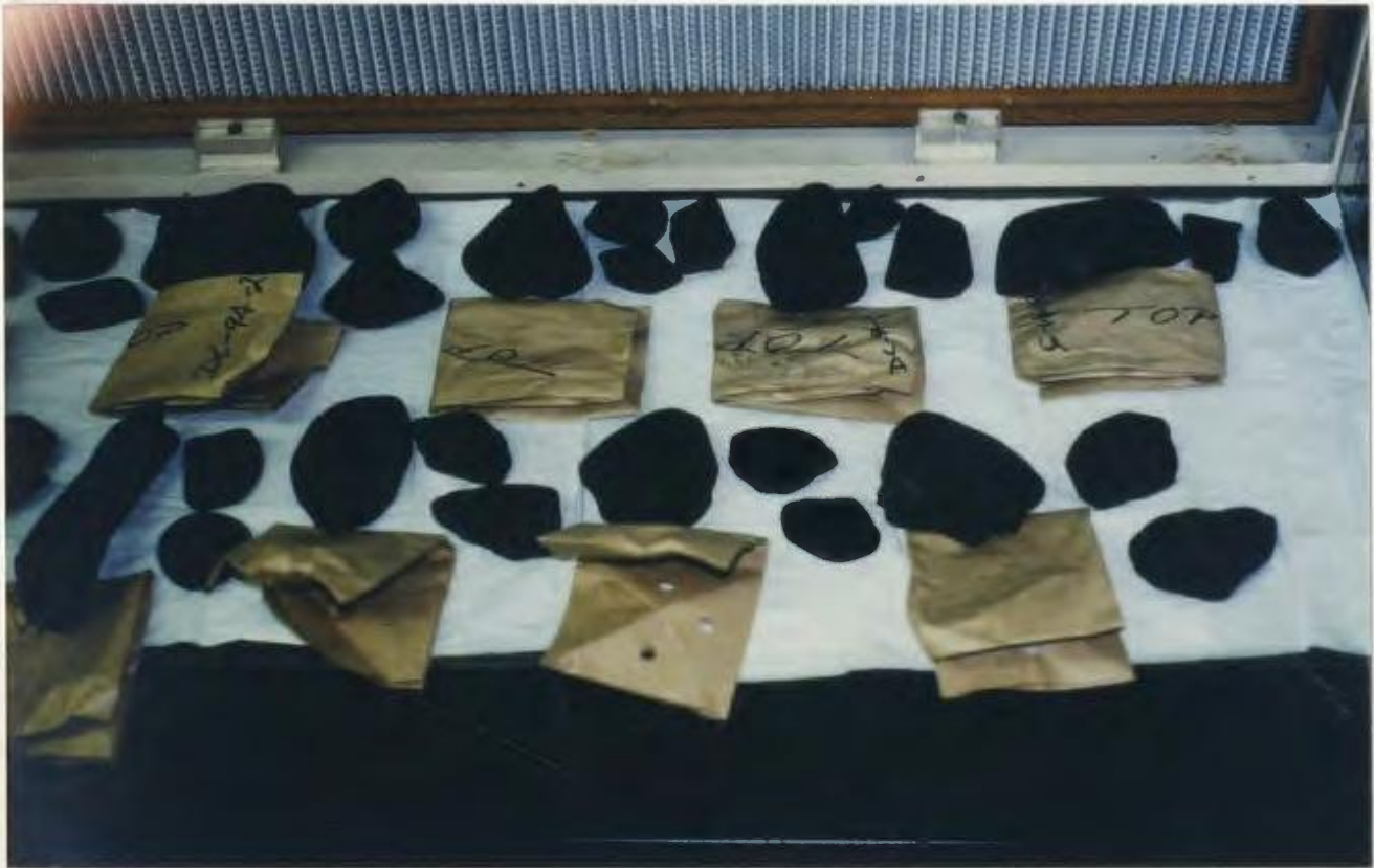
Plate 2.2: Filtered air drying of stream pebbles after cleaning with deionized water.
