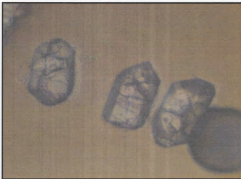
Plate 4-1: Transmitted light image of zircons from the silica-sericite-chlorite altered granite. Grains are less than 10 microns in length.
