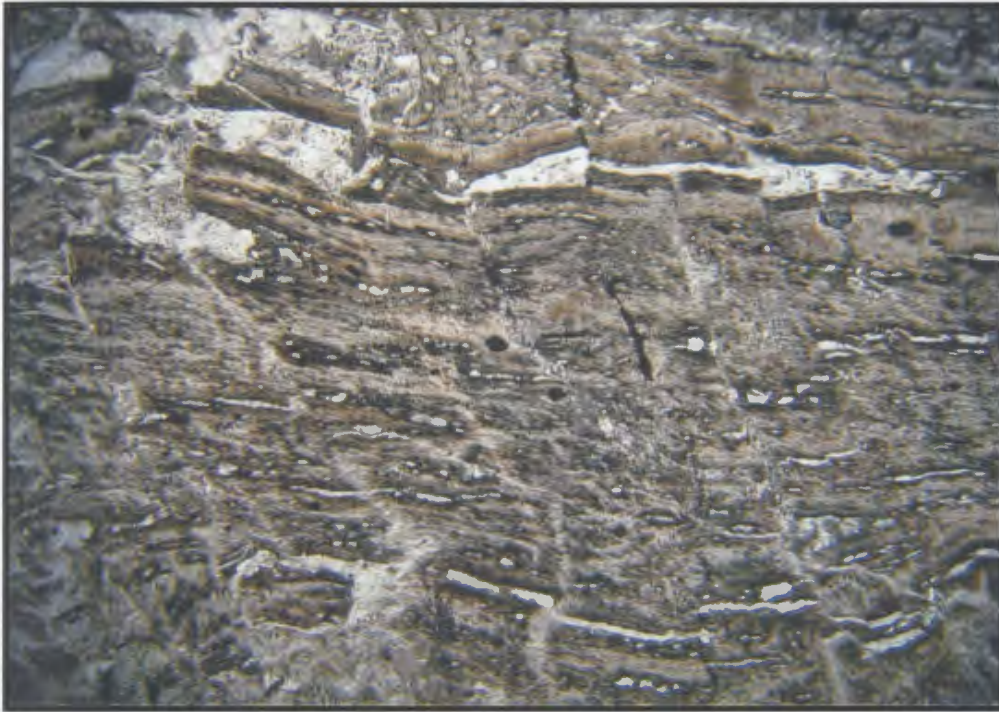
Plate 2-7: Photomicrograph of relatively uncompacted fiamme-bearing ash-flow tuff (CBS By-Pass roadcut; OB-01-011; PPL; FOV ~ 4.5mm).
