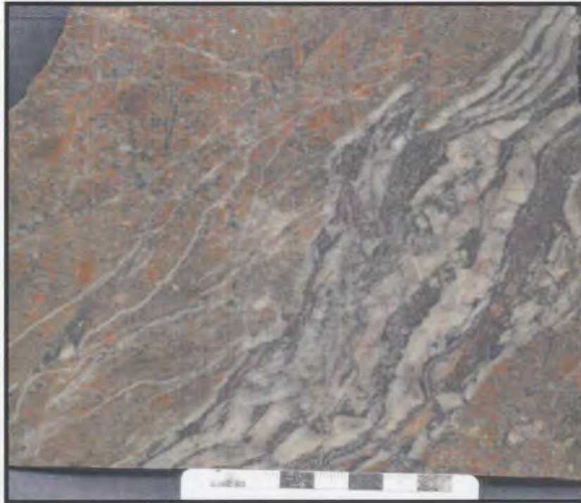
Plate 2-5: Lithic-rich, polymict lapilli tuff dominated by dark orange, potassic altered detritus. Note the unit is crosscut by banded chalcedonic silica-hematite veins of a low-sulphidation origin (Steep Nap prospect; scale is in cm).
