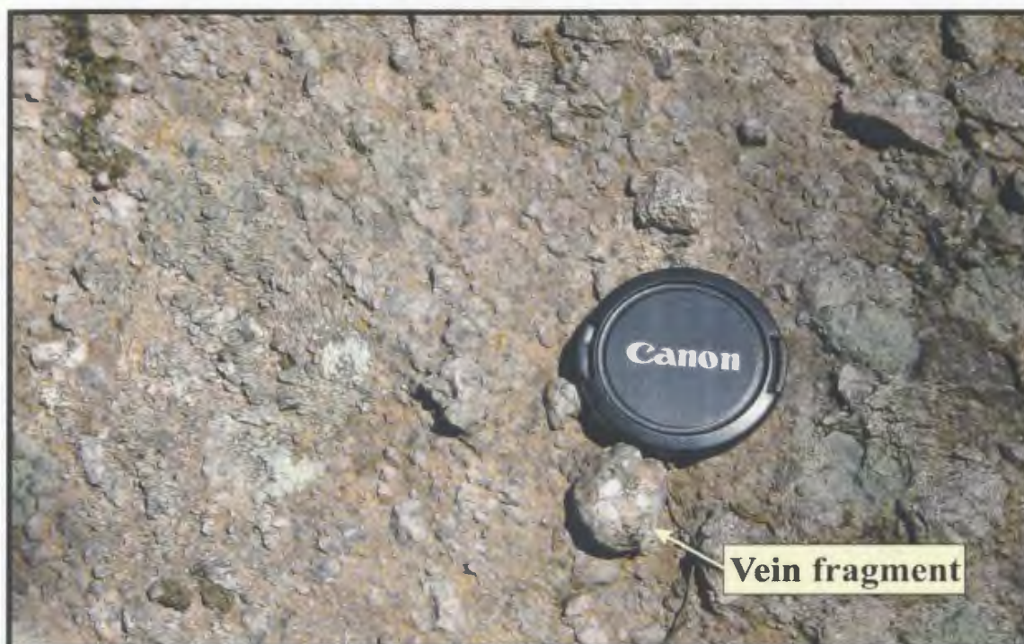
Plate 2-25: Hydrothermal eruption breccia containing fragments of chalcedonic silica-hematite vein material; clasts locally contain up to 7.75g/t Au (Bergs prospect; Photo courtesy of Sean O'Brien, Department of Natural Resources, Geological Survey).
