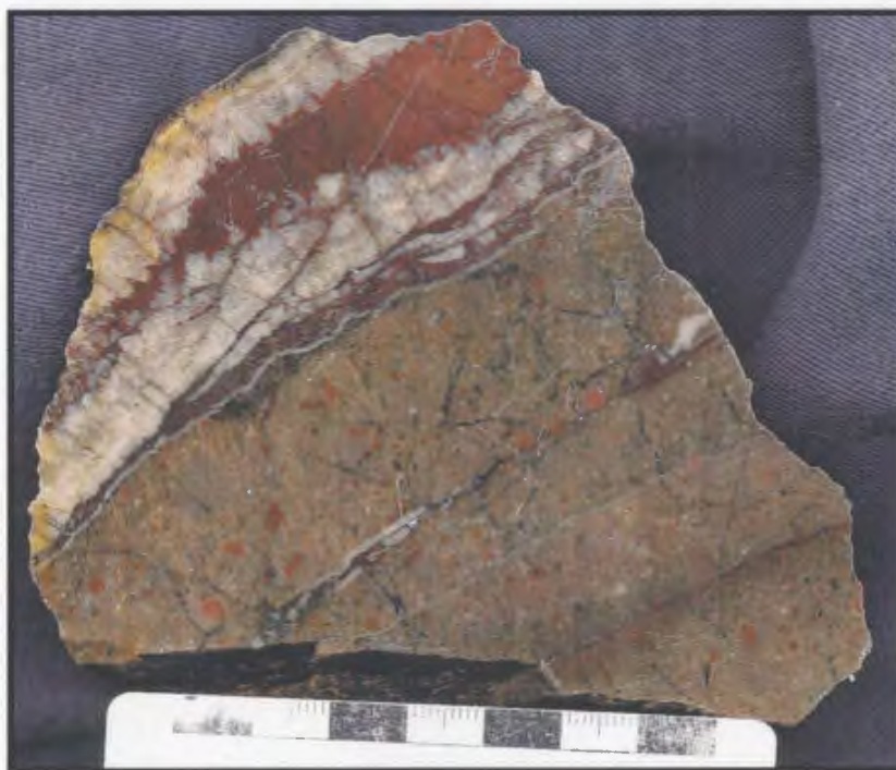
Plate 3-2: Representative hand sample of Unit 3 (Steep Nap prospect). Sample is crosscut by low-sulphidation-related quartz-hematite veins.
