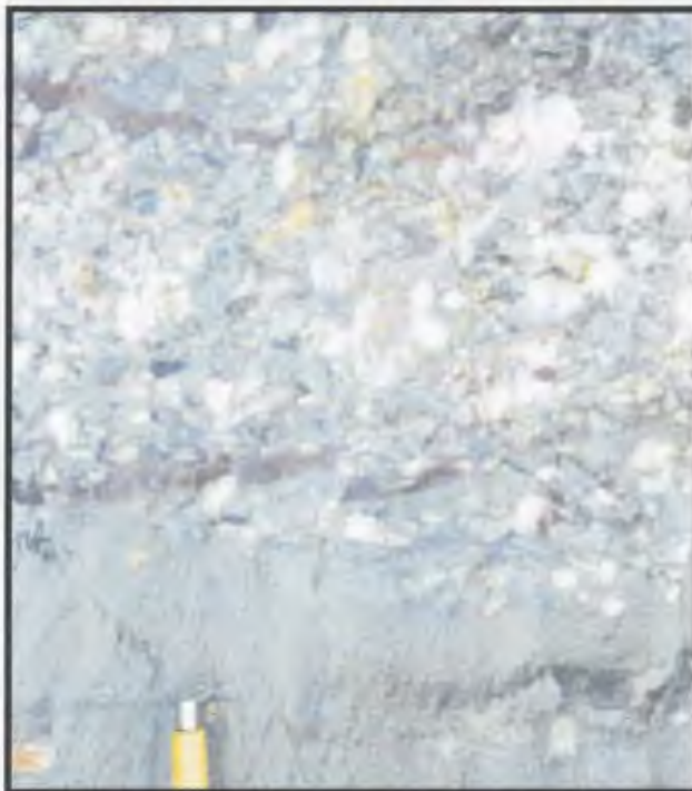
Plate 2-28: Basal conglomerate of Unit 19a (Oval Pit mine). Note the detrital silica-sericite alteration (white clasts) within the pebble conglomerate.
