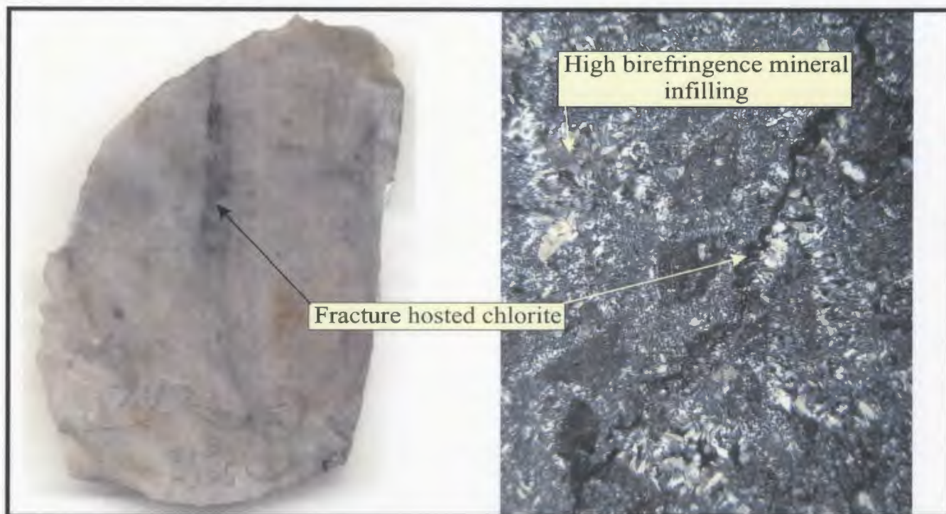
Plate 5-1: Thin section chip and associated photomicrograph of sample GS-03-101A, collected at vein margin (Trench #3). The thin section chip is 2.7cm wide; photomicrograph in XPL, FOV ~4mm. Note the high birefringence mineral in upper left hand corner of photomicrograph and abundance of silica in the matrix of the chip sample.
