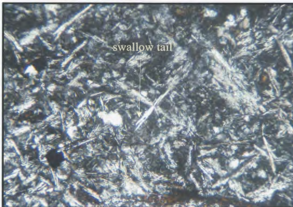
Plate 2-19: Photomicrograph of a swallow-tail texture developed in a mafic intrusion within Unit 7 of the White Hills Intrusive Suite (Bergs prospect); note texture implies rapid cooling (GS-02-061; XPL; FOV ~1mm).
