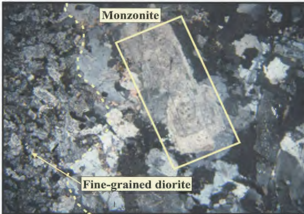
Plate 2-11: Photomicrograph of the contact between a diorite xenolith and Unit 6. The dashed line represents the approximated contact; note the subhedral plagioclase with preferential saussuritization of the central portion of the crystal outline in the rectangle (GS-02-81; XPL; FOV ~6mm).
