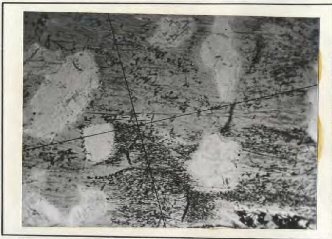
Fig. 15 Poikilitic texture in perknite. Sample taken at location J-12. Photomicrograph shows oikocrysts of hornblende enclosing chadocrysts of pyroxene. Hornblende also contains trains of magnetite inclusions. X 100 (approx.). Crossed nicols.
