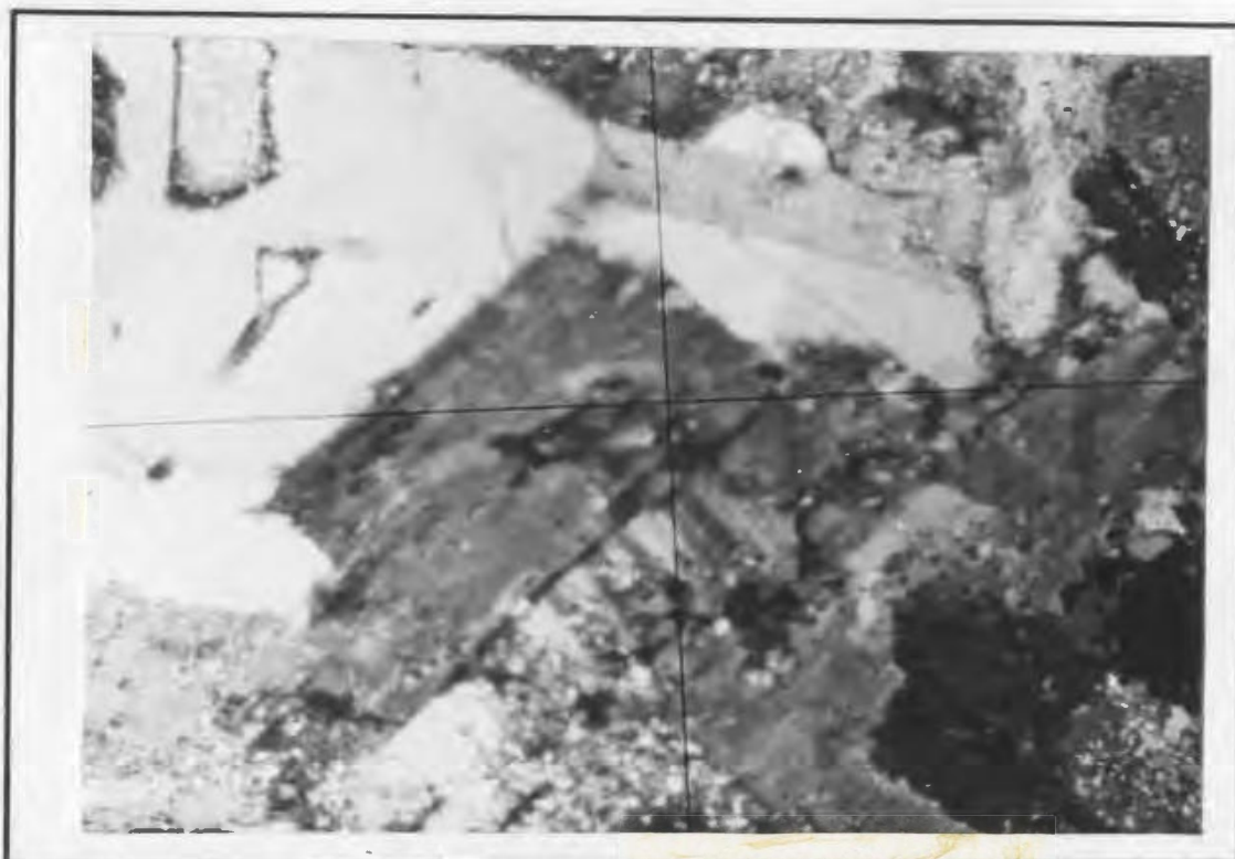
Fig. 4 Quartz diorite from location L-13. This rock is often gradational with more acidic types. Alterations are common. X 100 (approx.). Crossed nicols.
