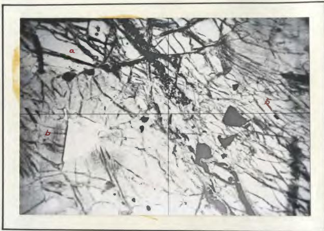
Fig. 9 Lherzolite taken within location E-8. Photomicrograph shows olivine (a), clino-pyroxene (b), and magnetite which fills cracks in olivine. X 65 (approx.). Crossed nicols.
