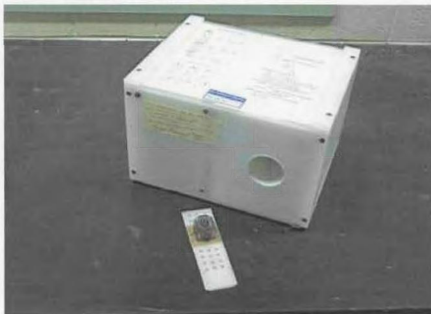
Figure 2.9 Sapphire Instruments (model SI2B) magnetic susceptibility meter. (Note the sample in the plastic holder in front of the instrument.)
