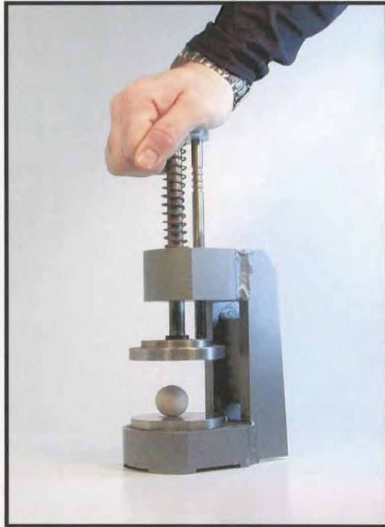
Figure 3.1 The non-magnetic press used to plastically deform sediment samples.
