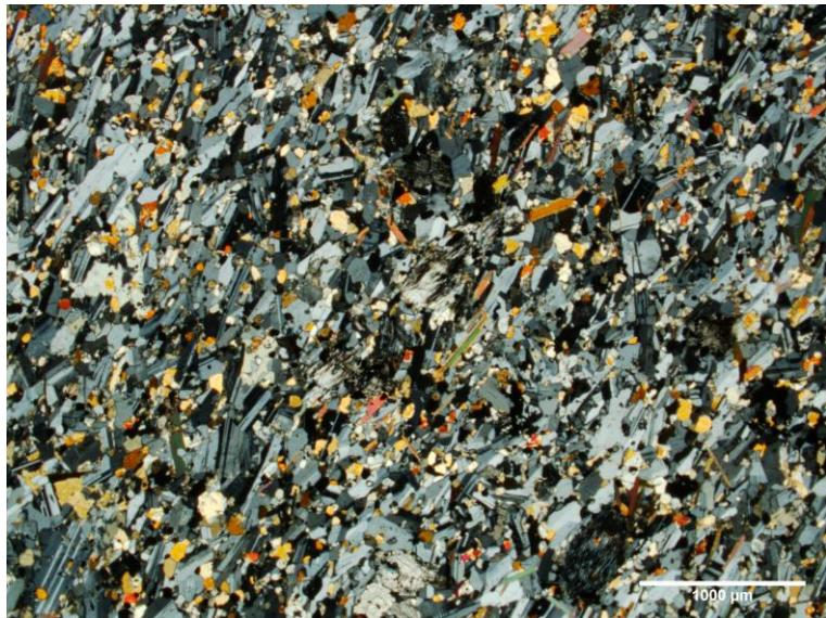
**Fig. 2-8.** Chilled gabbro from the Eastern Deeps (JG-11-101). This chill displays overall inequigranular texture with ragged, slightly elongate plagioclase laths and very fine pyroxene grains. The weak alignment of individual grains is possibly due to flow banding.
