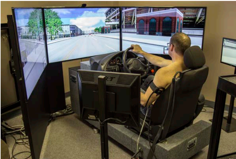
Figure 2. Participant in the Virage Simulator. The three large screens give a full frontal view similar to that of a windshield and the two small screens mimic the blind spots found while driving a motor vehicle.
